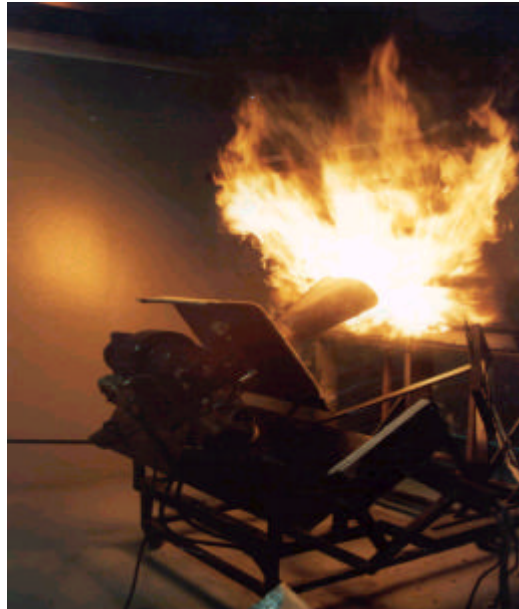
Figure 1. Burn-through apparatus and the flame it generated .
