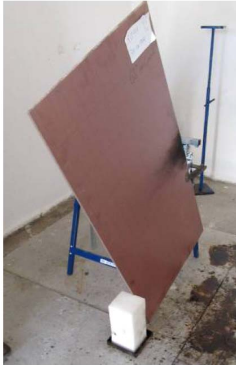
Potted edge after test (fire retardant potting compound)
