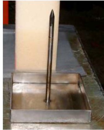
Figure 5.3.3.8-2 - Steel Tray with Pointed Steel Rod
