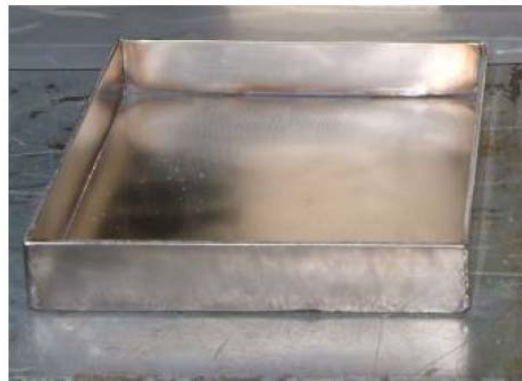
Figure 5.3.3.8-3 - Steel Tray Used for Soaking Bottom of Foam Block with Heptane
