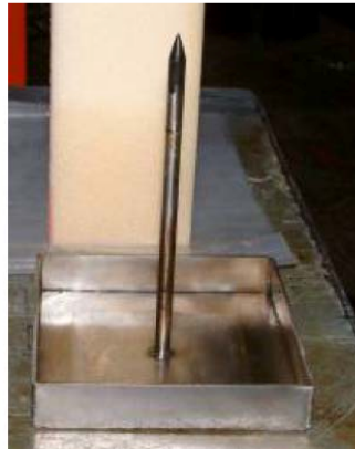
Figure 5-2 - Steel Tray with Pointed Steel Rod
