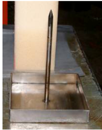
Figure 5.3.3.8-7 - Steel Tray with Pointed Steel Rod
