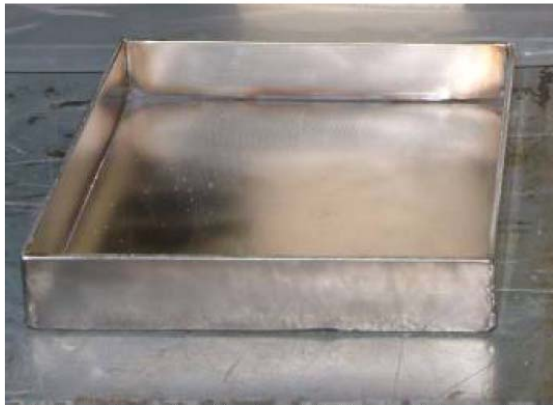
Figure 5-3 - Steel Tray Used for Soaking Bottom of Foam Block with Heptane
