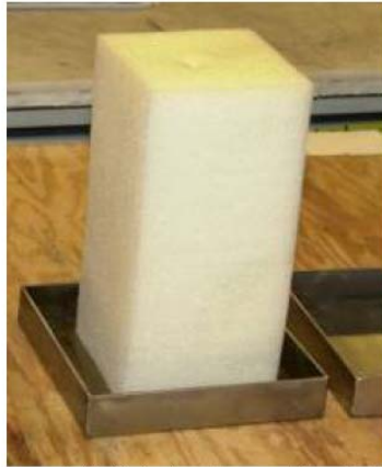
Figure 5.3.3.8-1 - Foam Block Fire Source
