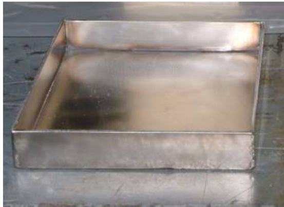
Figure 5.3.3.8-8 - Steel Tray Used for Soaking Bottom of Foam Block with Heptane
