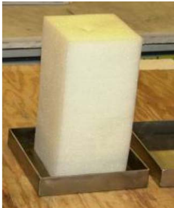
Figure 5-1 - Foam Block Fire Source
