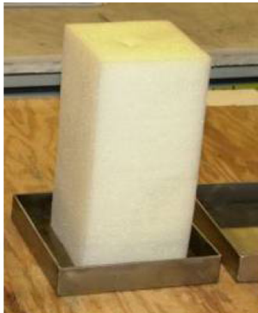
Figure 5.3.3.8-6 - Foam Block Fire Source
