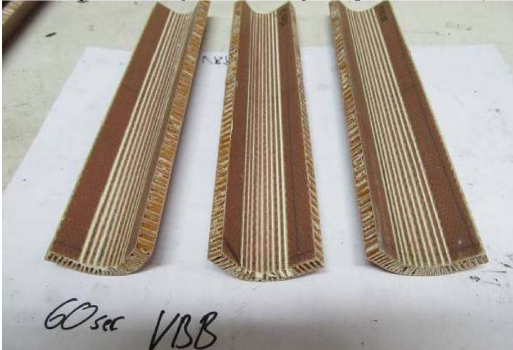
Photo of Sample K-0415: multiple ditch 1" Radius after 60sec VBB testing (worst case adhesive) Flame has been extinguished after 120 seconds intentionally
