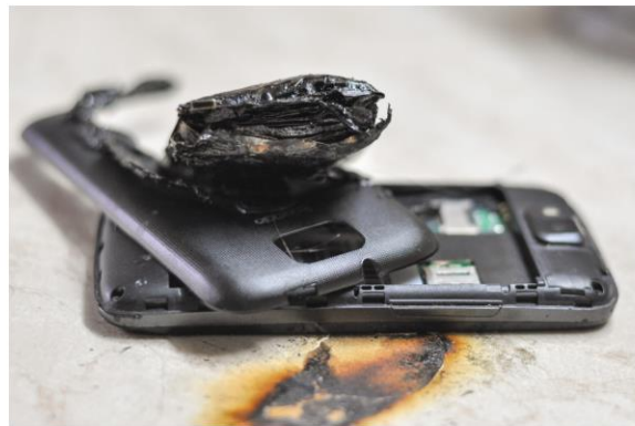
Smartphone battery after Thermal Runaway. © Adobe Stock
