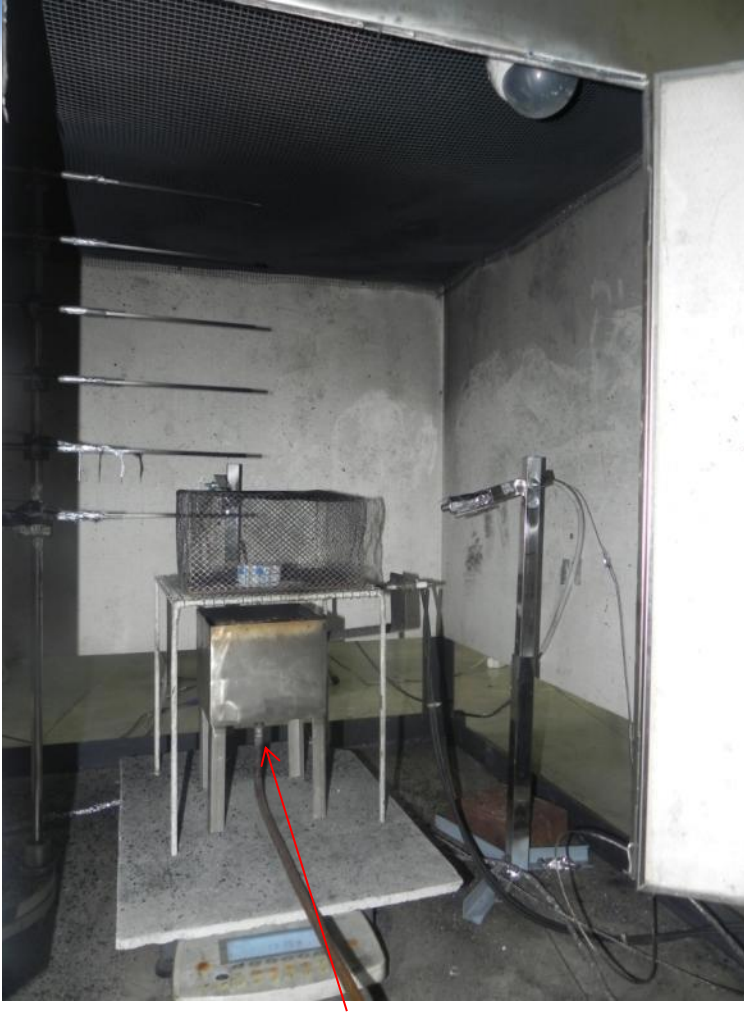
Flame Exposure: Propane heater
