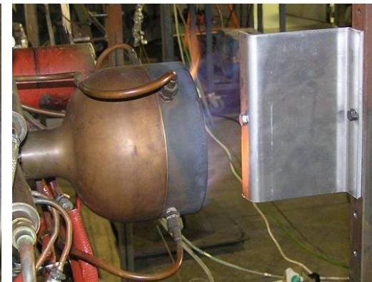
➤ Former and bolt (simulating the critical part)
