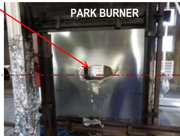
Large burnthrough on the centerline
