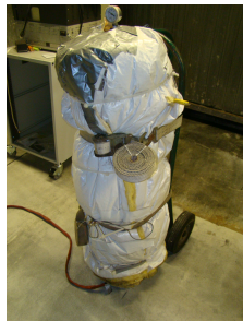
Vent Gas Storage Tank
