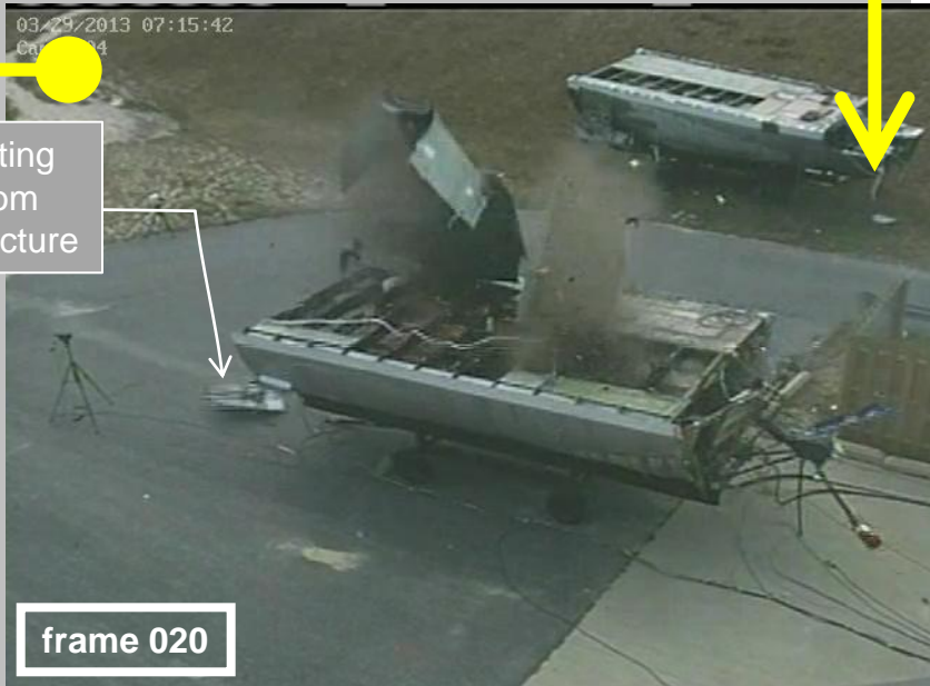
note transient skin flexure at floor beam plane
