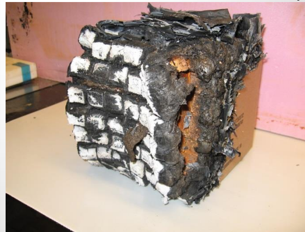
Post Test Packing fuses to form a protective barrier.
