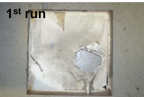
30° , 9m10s & 9m30s surface melted
