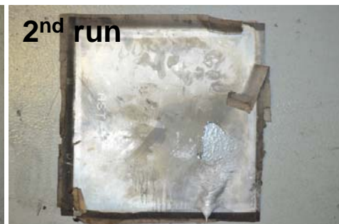
30° , 9m10s & 9m30s surface melted
