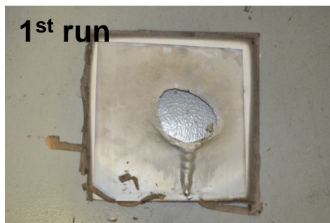
45° , 10m & 9m40s surface melted
