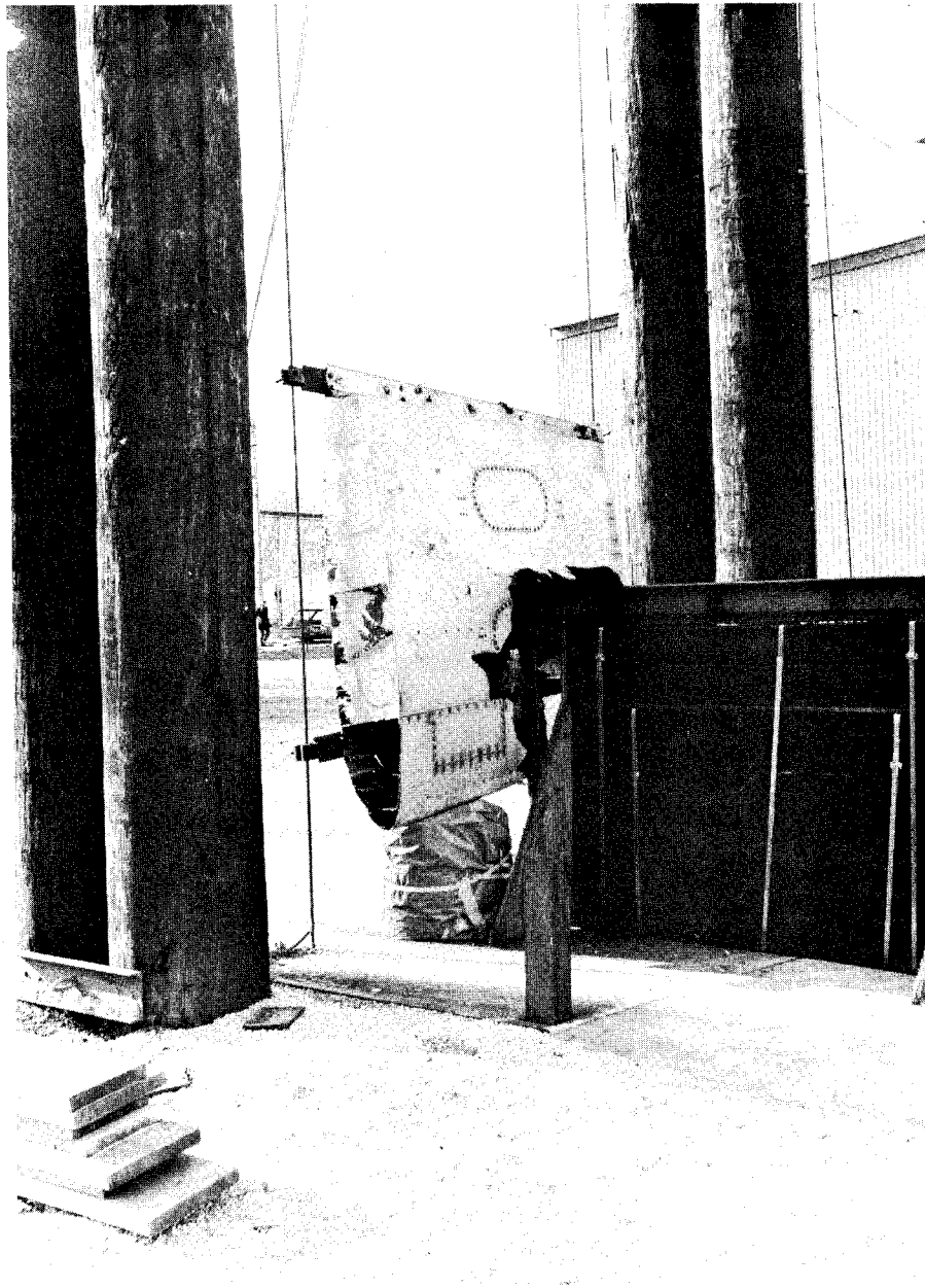
FIGURE 4 DROP TOWER SLASHING TEST ON DC-7 WING TANK SECTION
