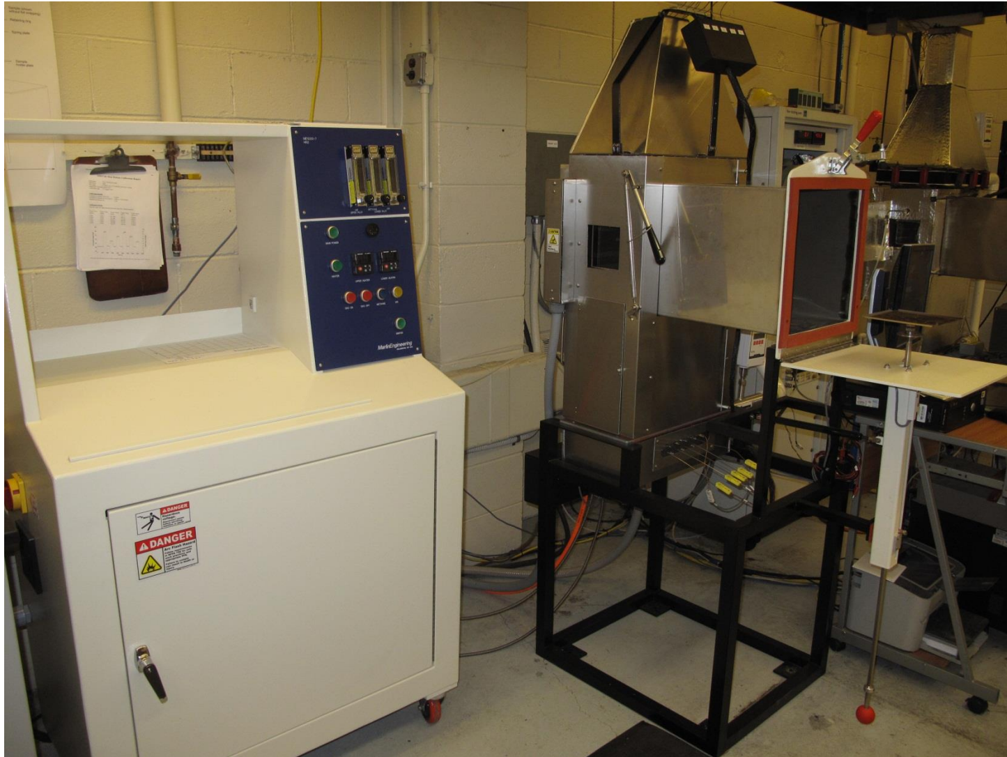
Heat Release Rate Test Apparatus October 2014
