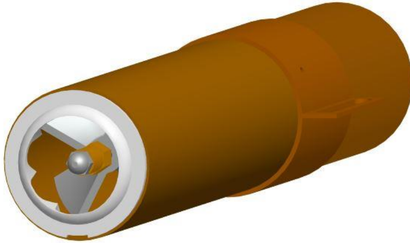
Figure 8-S-17. Position of Turbulator at the end of the Draft Tube
