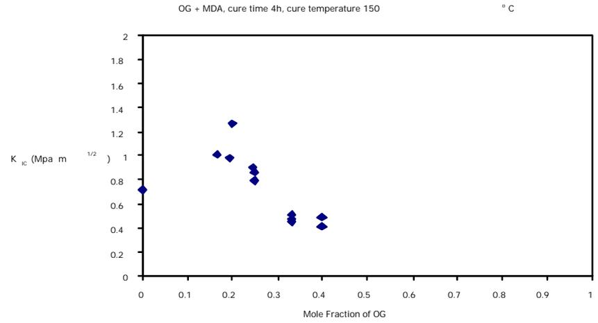
**Figure 4. Fracture Toughness of OG/MDA Epoxy** Data point at 0 MF OG is for DGEBA/MDA
