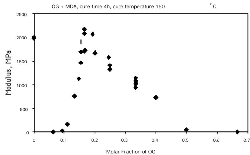
Figure 3. Elastic Modulus of Epoxy Resin Made with Octaglycidyl Octasilsesquioxane (OG) and Dianilinomethane (MDA).
