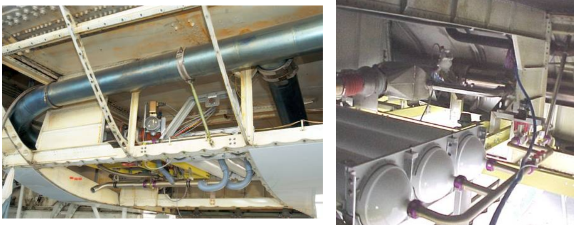
Figure 4. The FAA OBIGGS Installed on NASA B-747 SCA
