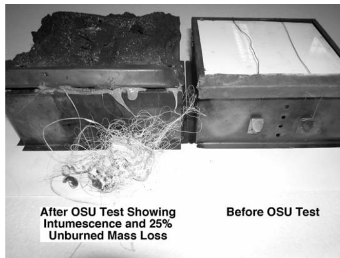
Figure 7. White Polyestercarbonate Before and After 14 CFR Part 25 Testing for HR in the OSU
