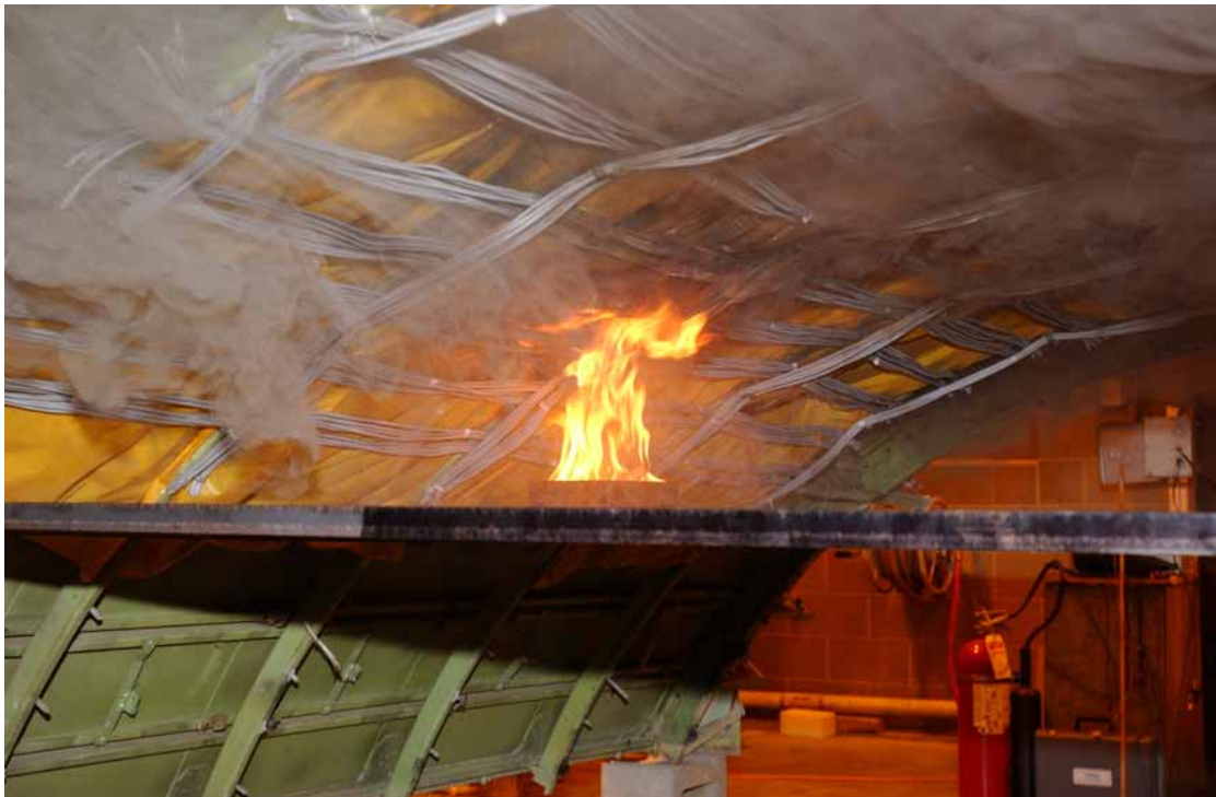
FIGURE 18. TEST PROGRESSION OF RISER CABLE (A), VIEW 1
