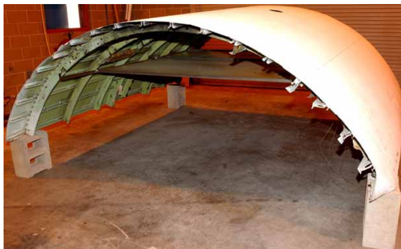
FIGURE 2. INTERMEDIATE-SCALE WIRE TEST ARTICLE
