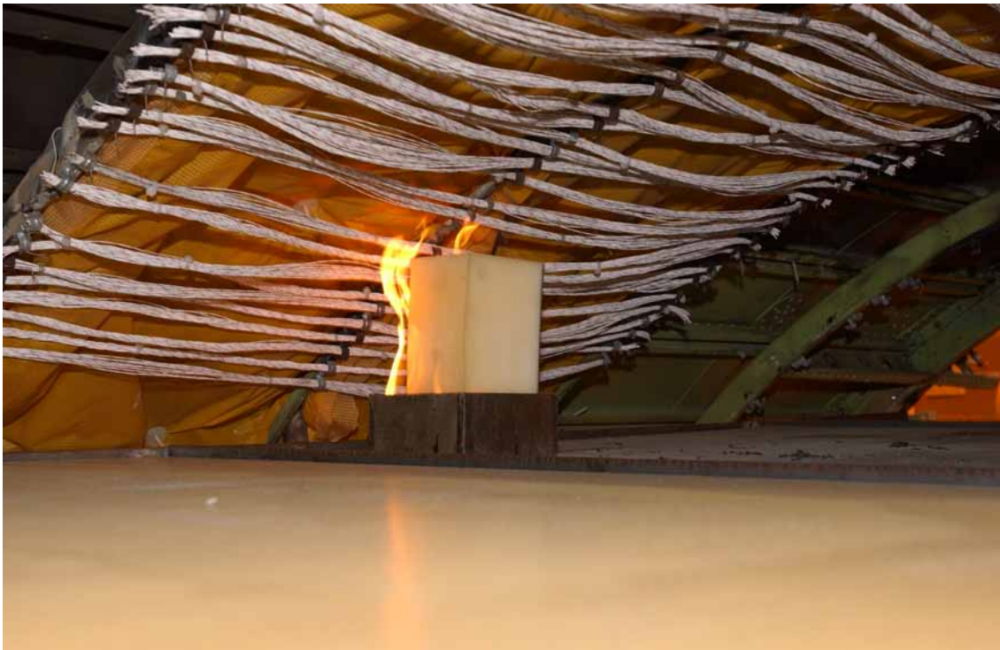
FIGURE 32. IGNITION OF PTFE/POLYIMIDE/PTFE
