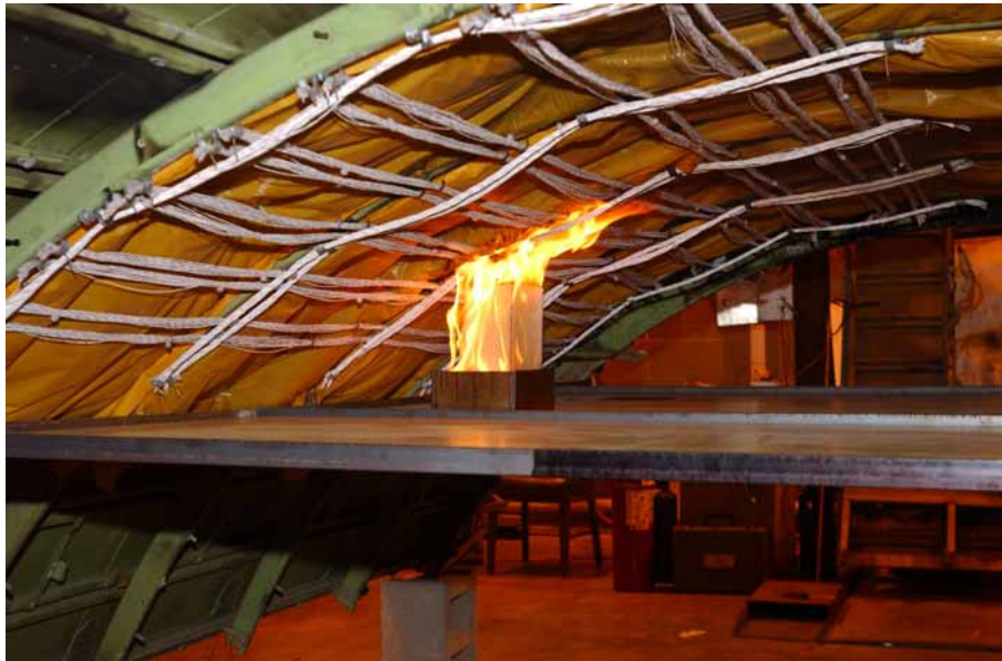
FIGURE 11. IGNITION OF PTFE/POLYIMIDE/PTFE
