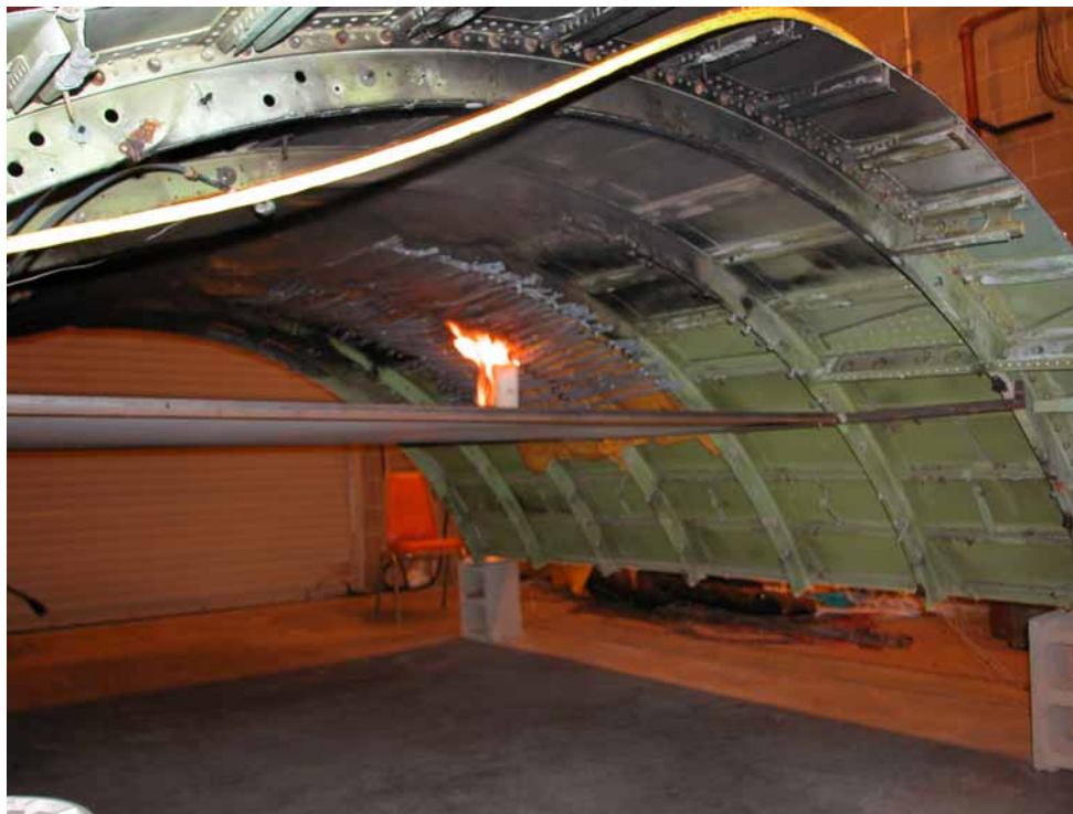
FIGURE 36. IGNITION OF RISER CABLE (A)
