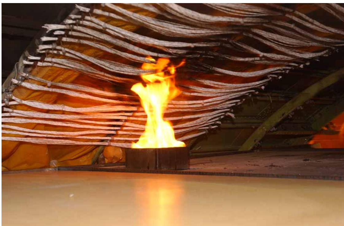
FIGURE 34. TEST PROGRESSION PTFE/POLYIMIDE/PTFE, VIEW 2
