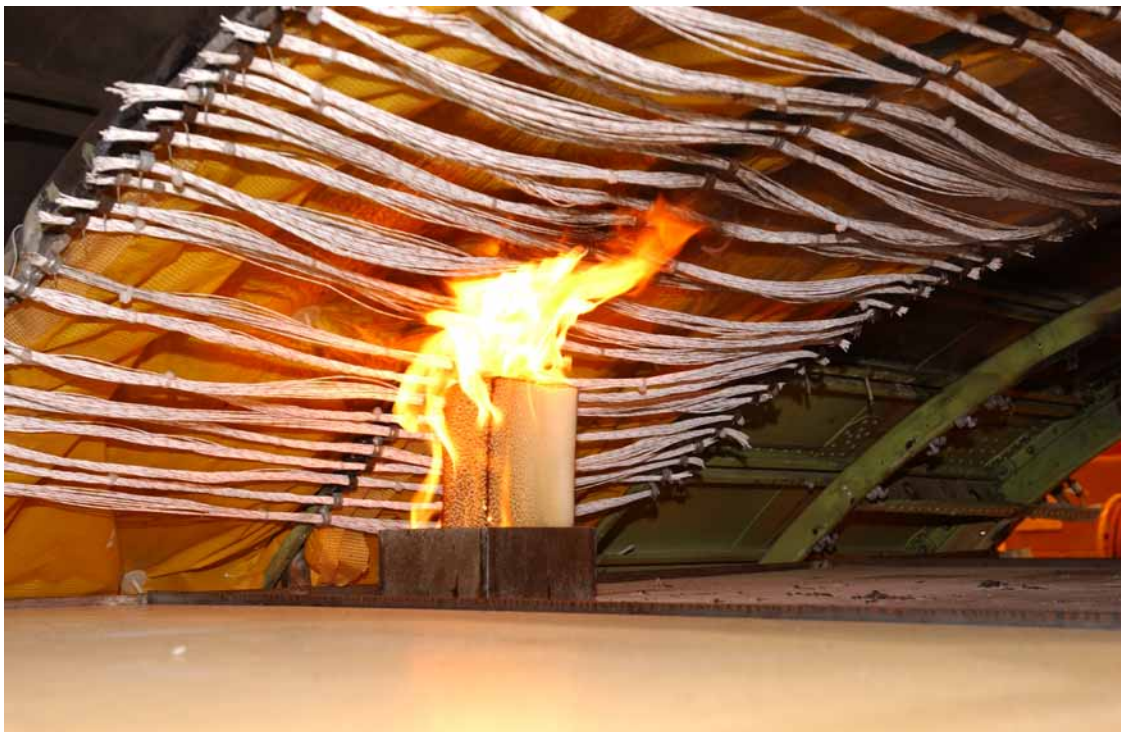
FIGURE 33. TEST PROGRESSION OF PTFE/POLYIMIDE/PTFE, VIEW 1
