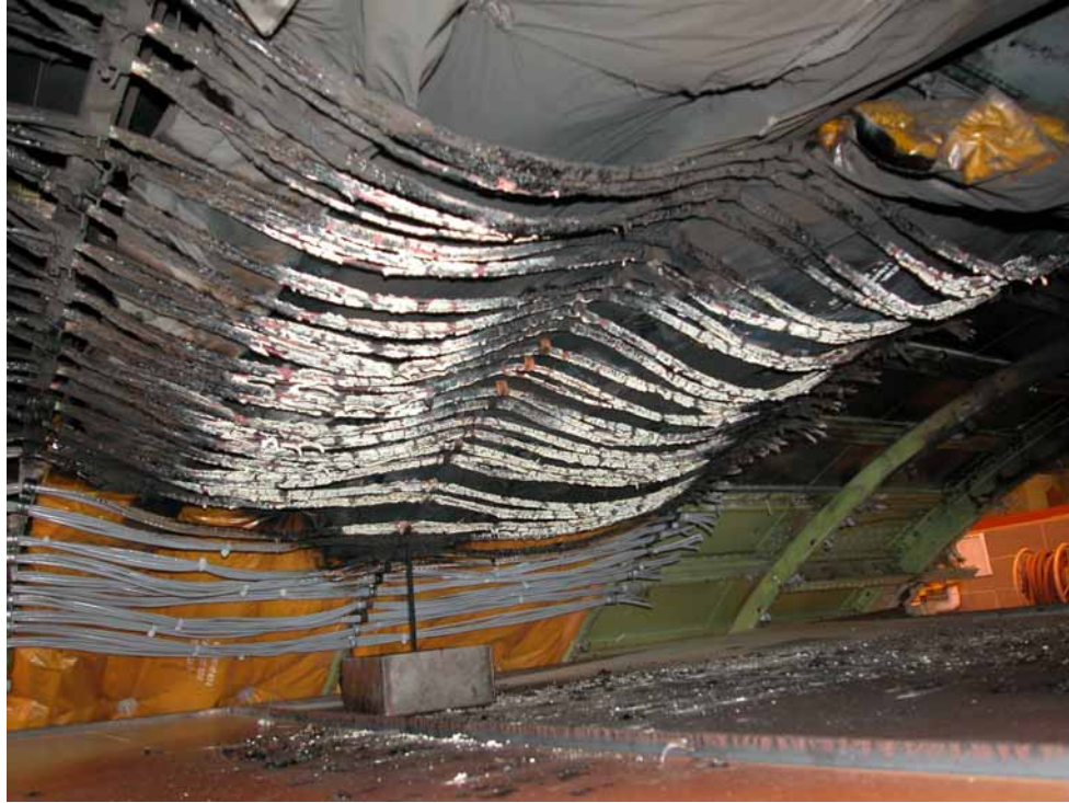
FIGURE 43. FLAMEOUT OF RISER CABLE (A), CROSS VIEW
