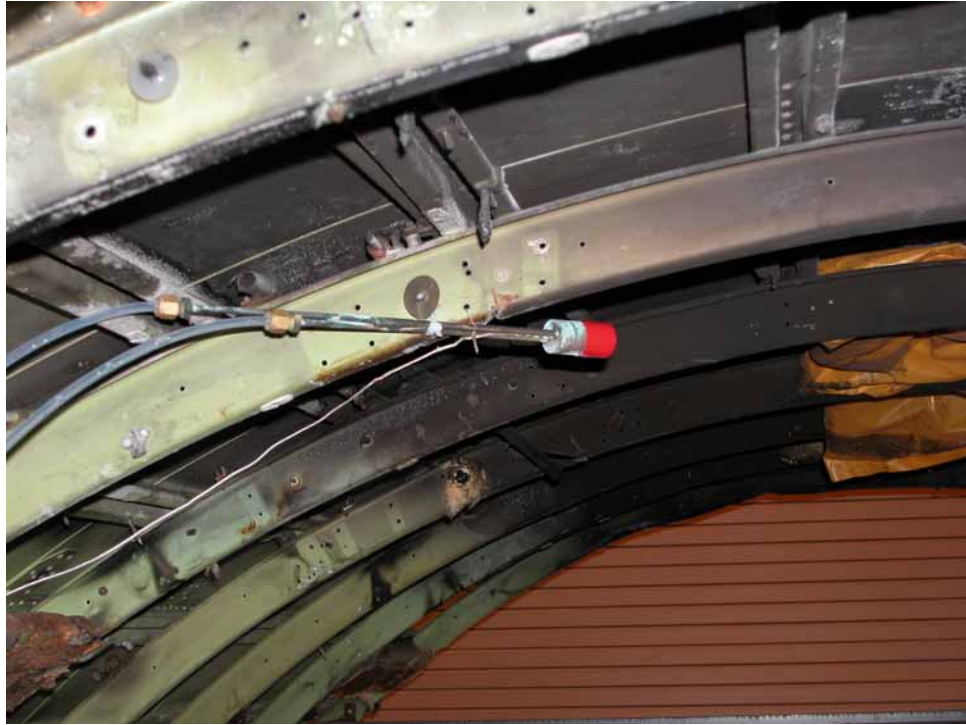
FIGURE 4. GARDON GAUGE PLACEMENT
