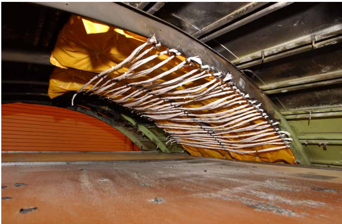
FIGURE 29. INTERMEDIATE-SCALE CABIN ATTIC FLAMMABILITY TESTS CONFIGURATION 2
