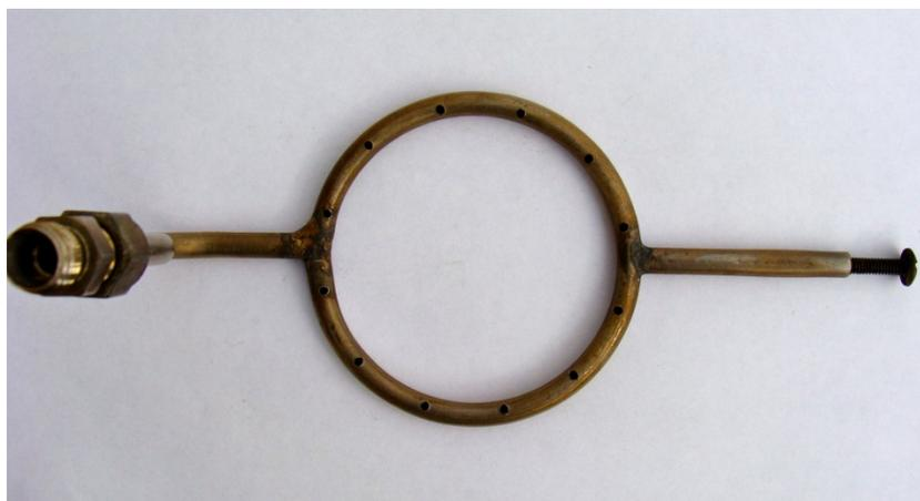
**Figure 1. Exhaust gas sampling ring**
