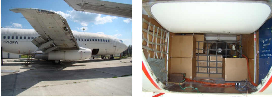
Figure 2. The 737 forward cargo compartment
