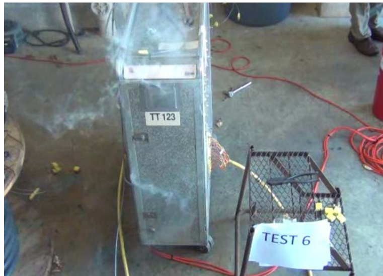
Figure 28. Thermal runaway event
