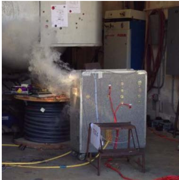
Figure 23. Thermal runaway event within the cart
