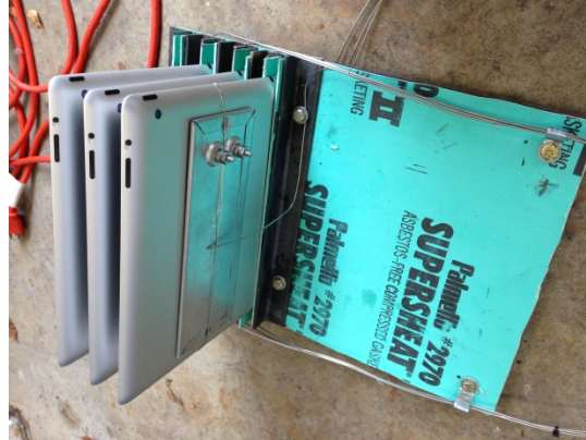
Figure 2. Test rig with 1-inch spacing
