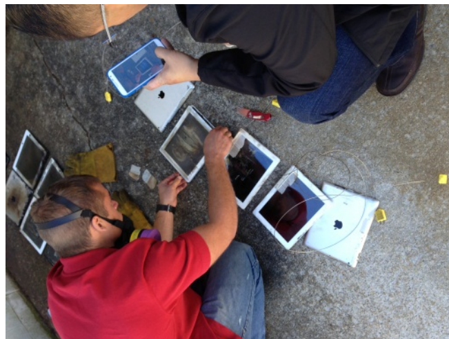
Figure 30. Disassembly of damaged e-tablets
