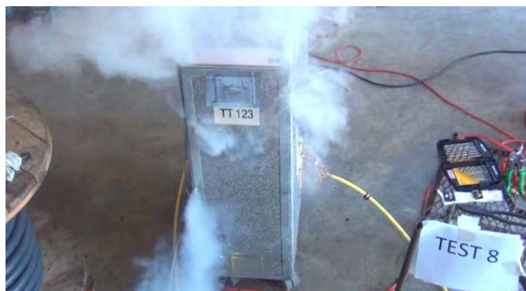
Figure 38. Test 8 thermal runaway event 3
