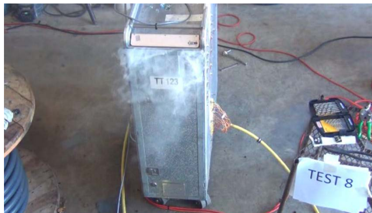
Figure 37. Test 8 thermal runaway event 2
