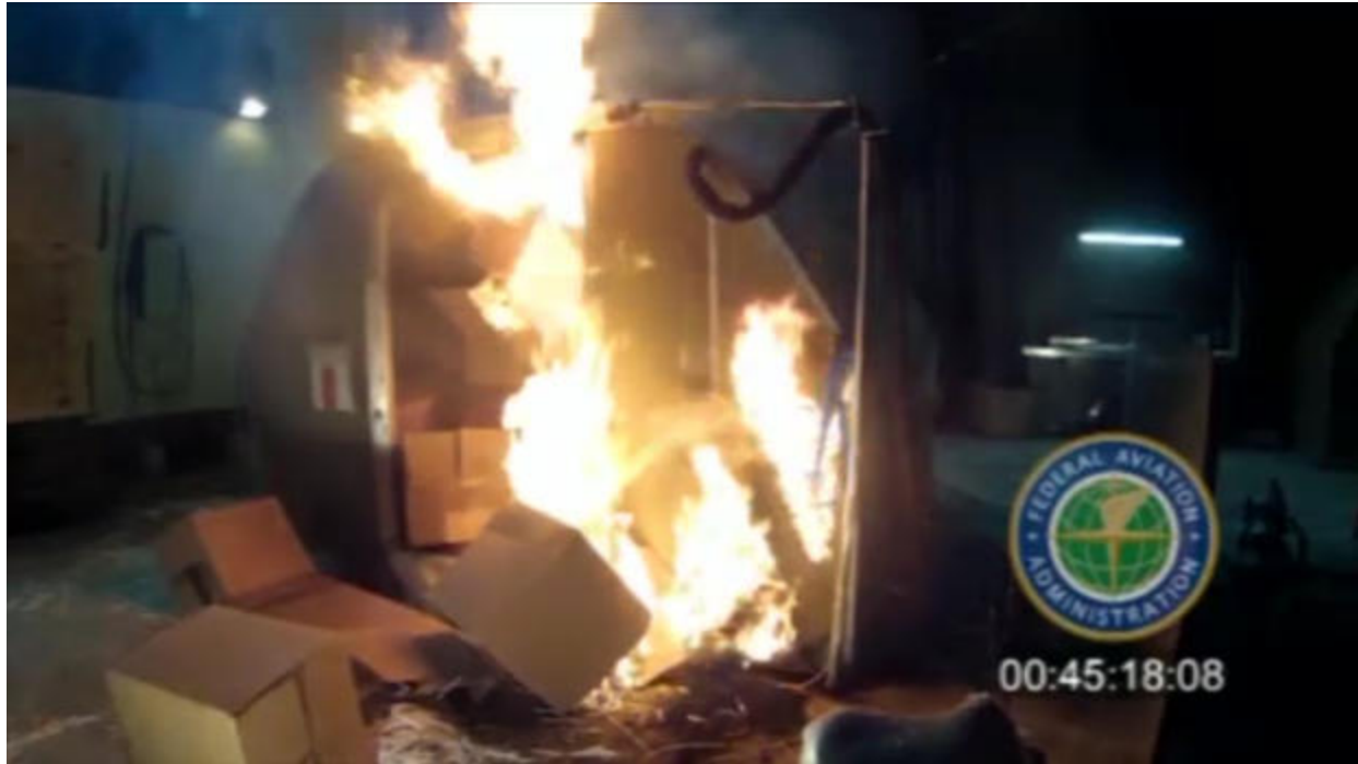
Figure 1. Cargo container explosion caused by lithium battery vent gases
