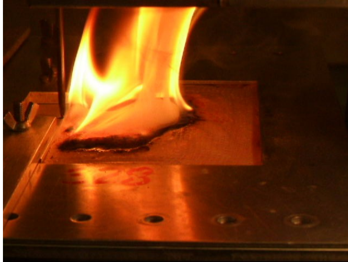
Figure 8. Hydraulic Fluid Fire During 200° C Test
