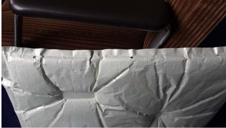
Figure 34. TAI Drainage Holes (bottom edge view)
