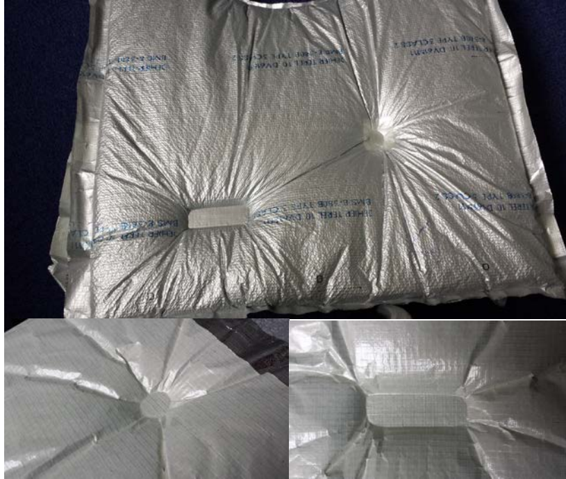
Figure 36. Thermal Weld Showing Provision for Apertures to Be Cut
