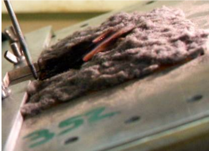
Figure 7. Flame Propagation (dust and lint contamination level 80 grams/m 2 )
