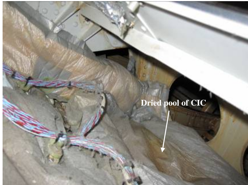
Figure 19. Localized Area of CIC Contamination on TAI
