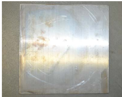
Figure 38. Test Sample After 20 Minutes of Propane Burner Operation
