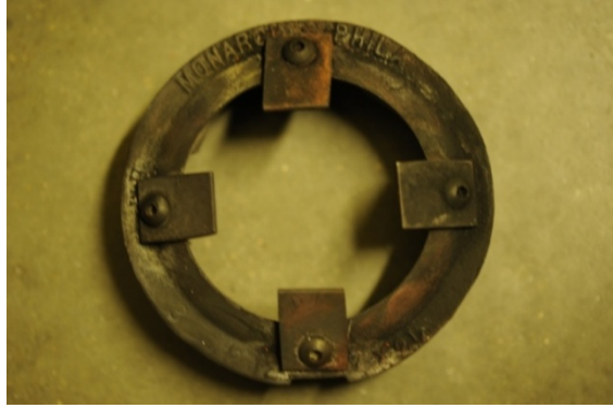
Figure 3. Modified Monarch F-124 Turbulator With Four Tabs
