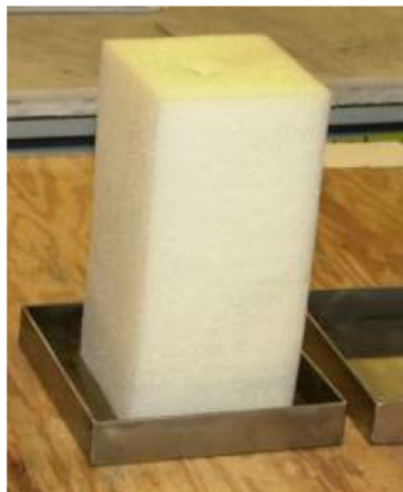
Figure 5.3.3.8-6 - Foam Block Fire Source
