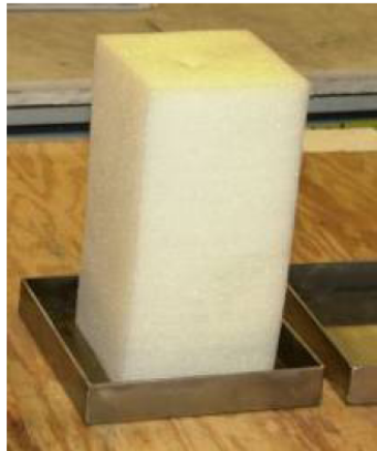
Figure 5-1 - Foam Block Fire Source
