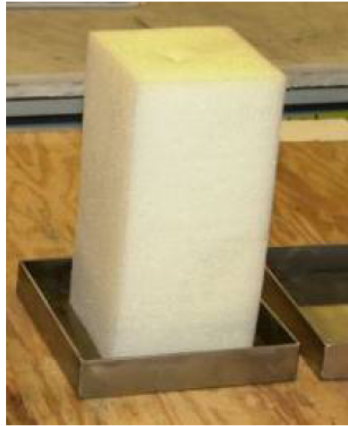
Figure 5.3.3.8-1 - Foam Block Fire Source
