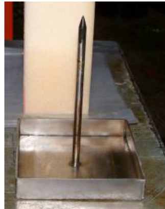
Figure 5-2 - Steel Tray with Pointed Steel Rod
