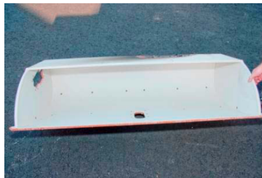
Inserts inside a stowbin for attaching trim
