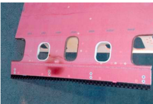
Inserts along a panel edge for attaching trim
