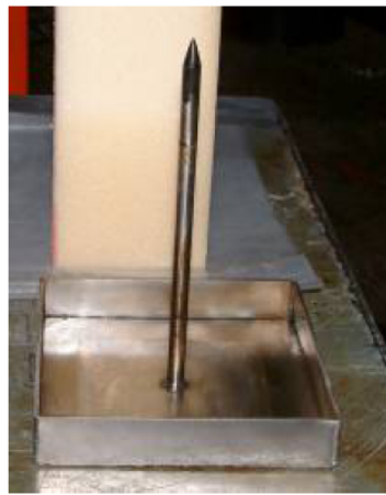
Figure 5.3.3.8-7 - Steel Tray with Pointed Steel Rod
