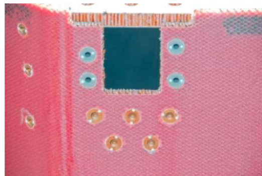
Inserts around a cutout for a fitting.
