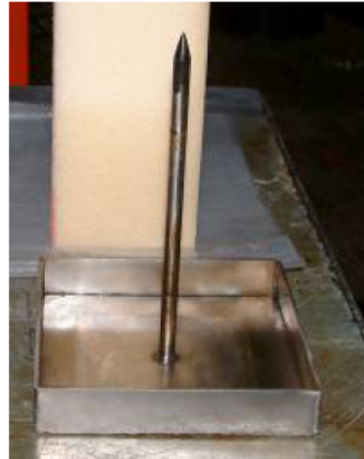
Figure 5.3.3.8-2 - Steel Tray with Pointed Steel Rod
