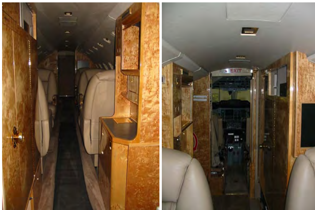
Figure 16. Galley & Luggage Compartment on Aisle Leading to Main Passenger Door (left: viewed from cockpit; right: viewed from cabin) (Airplane C)
