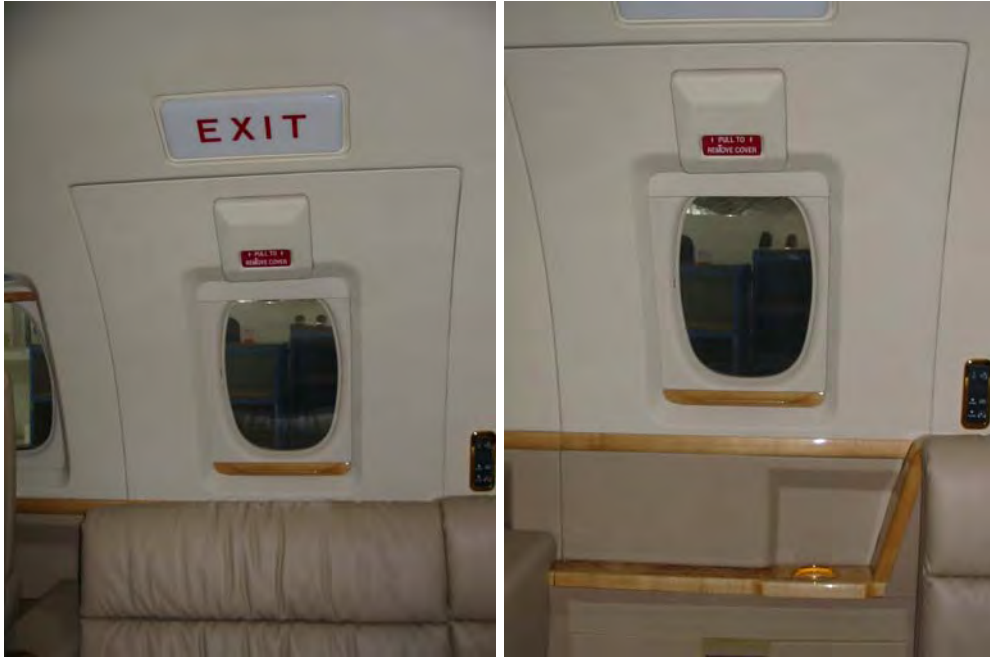
Figure 21. Type III Emergency Exit With Divan-Type Seat Fitted Underneath (Airplane C)
