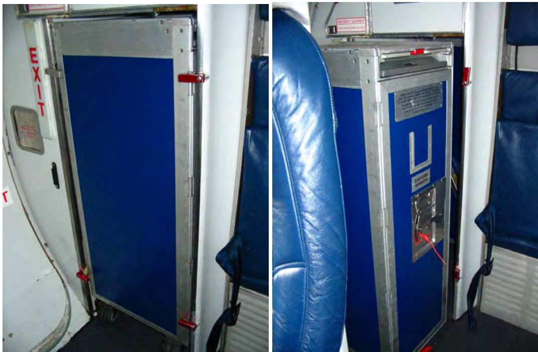
Figure 18. Galley at Right-Hand Aft Emergency Exit Area (left: cart stowed; right: cart loose and blocking the exit) (Airplane F)
