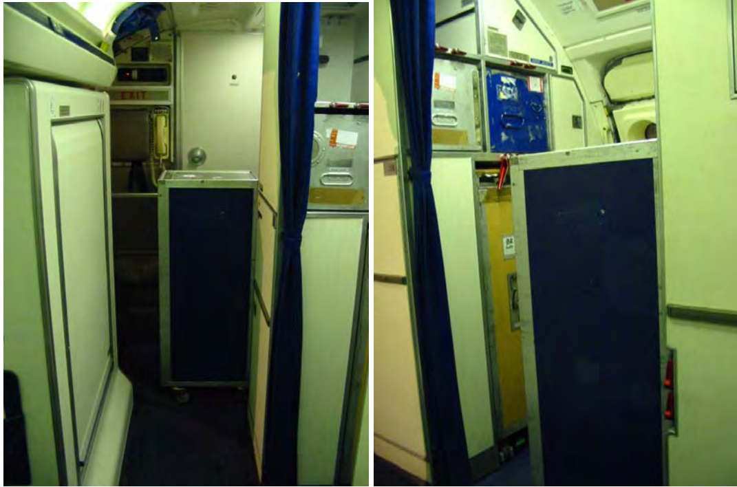
Figure 19. Passageway to Forward Left Emergency Exit (left) and Forward Right Emergency Exit (right)—Cart is Shown Dislodged (Airplane H)
