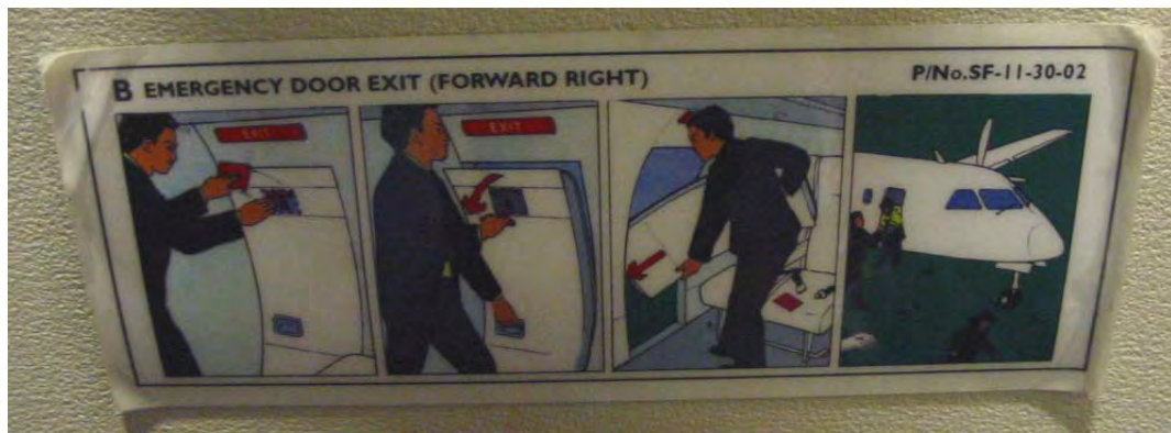
Figure 6. Type I Emergency Exit and Opening Instructions (Airplane G)
