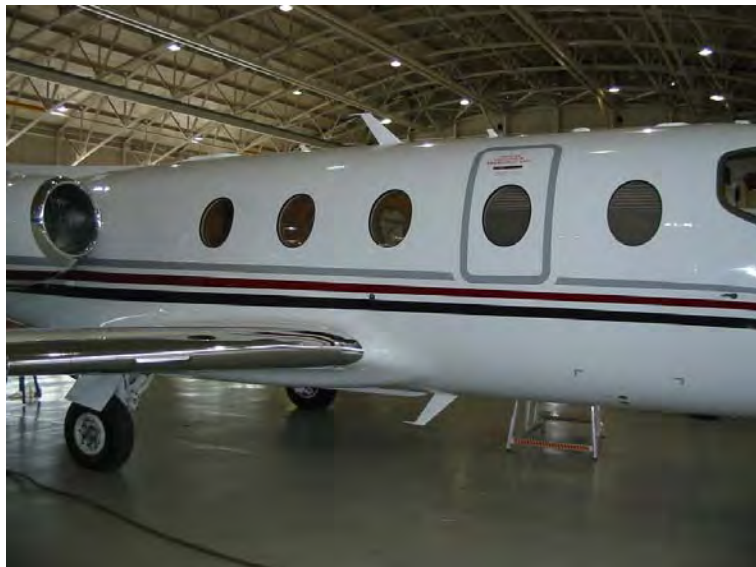
Figure 31. Type III Exit on Airplane A (exit height approx. 1.5 m/4.9 ft)
