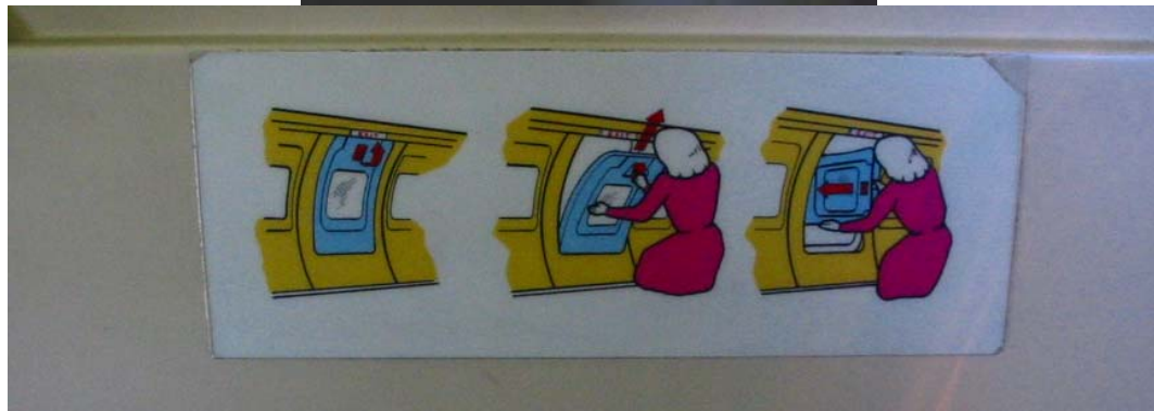
Figure 3. Type III Emergency Exit and Opening Instructions— Passenger Standing Up (Airplane D, similar to Airplane F)
