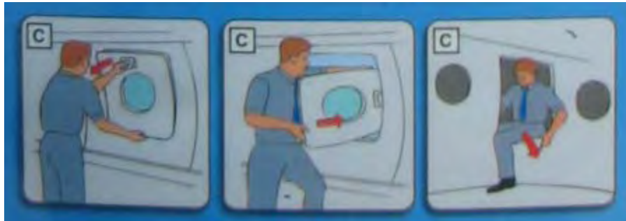
Figure 34. An Example of an Instruction to Exit From a Type IV Exit in the Safety Card (Airplane D)
