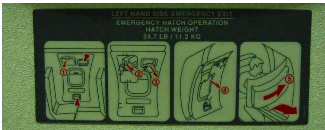
Figure 4. Type III Emergency Exit and Opening Instructions— Passenger Sitting Down (Airplane H)
