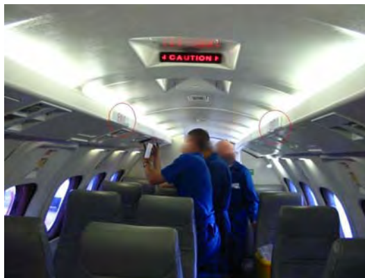
Figure 36. Overwing Exit Locating Signs on Airplane D—Not Above Aisle (circled)
