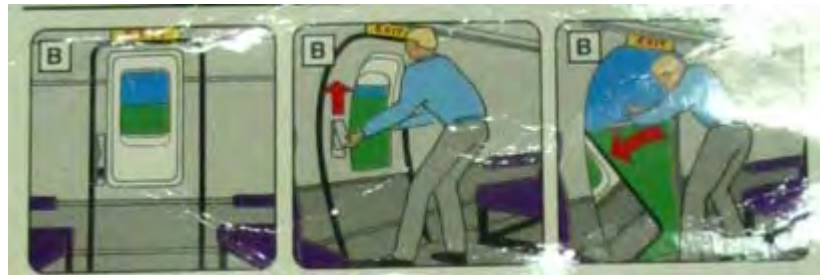
Figure 8. Type I Emergency Exit and Opening Instructions (Airplane I) – Hatch can be Pushed Out
