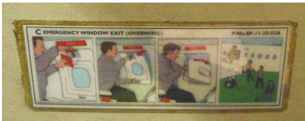
Figure 5. Type III Emergency Exit and Opening Instructions— Passenger Sitting Down (Airplane G)
