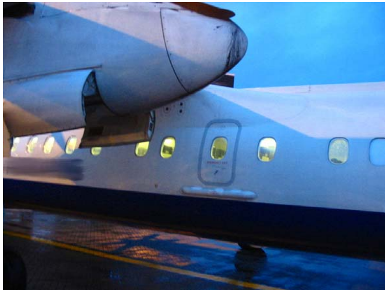
Figure 33. Type III Exit on Airplane I (exit height approx. 1.5 m/4.9 ft)
