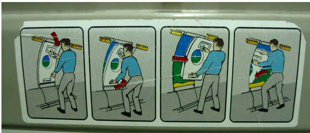
Figure 2. Type III Emergency Exit and Opening Instructions— Passenger Standing Up (Airplane I)
