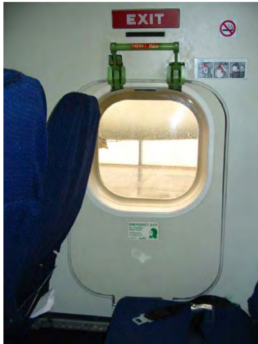
Figure 22. Minor Obstruction of Emergency Exit Window (Airplane E)
