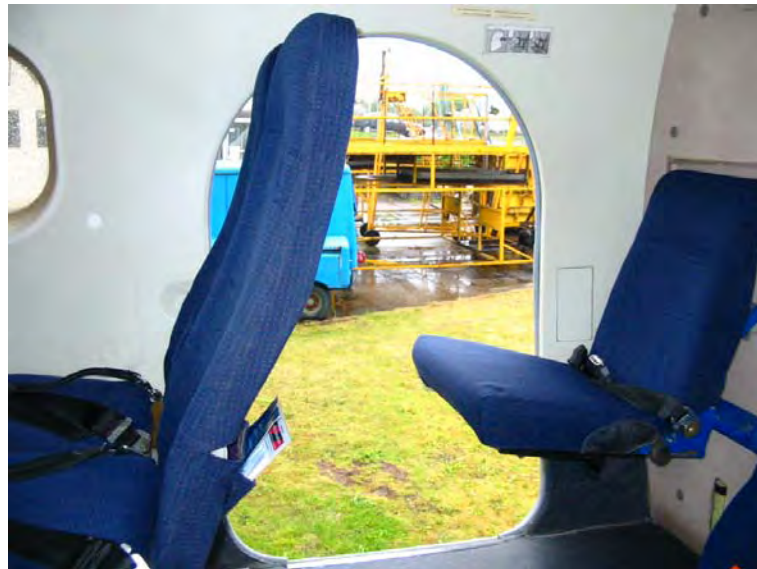
Figure 20. Aft Right-Hand Emergency Exit Obstructions (Airplane E)
