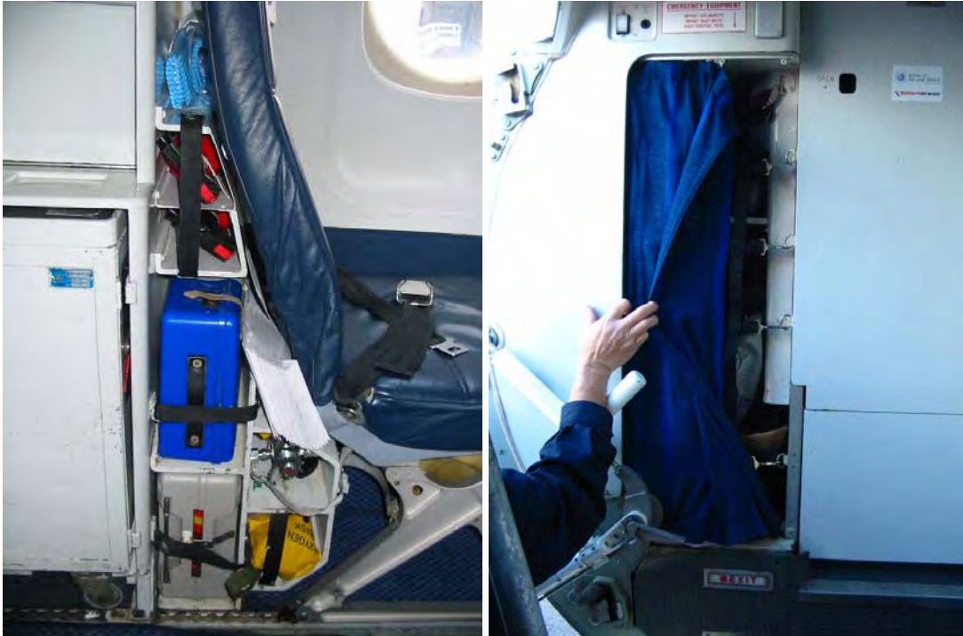
Figure 27. Emergency and Service Equipment Stowage (left: against rear bulkhead, right: behind front bulkhead) (Airplane F)
