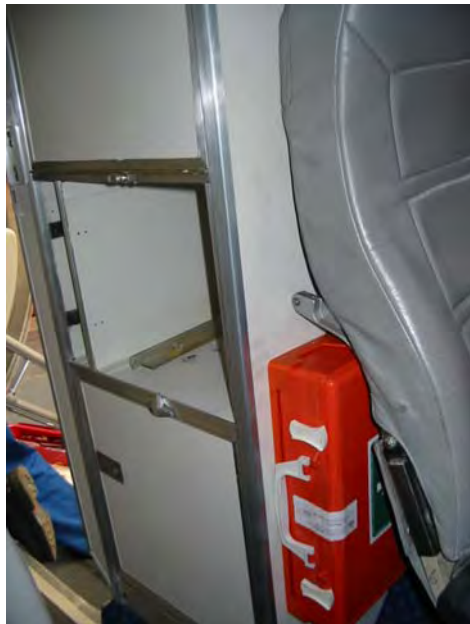
Figure 26. First Aid Kit Stowage (Airplane D)
