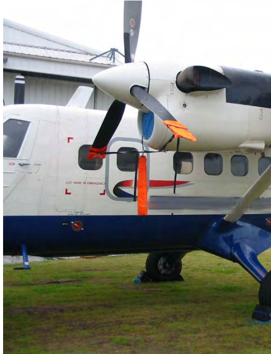
Figure 32. Type IV Exit on Airplane E (exit height approx. 1.75 m/5.77 ft)
