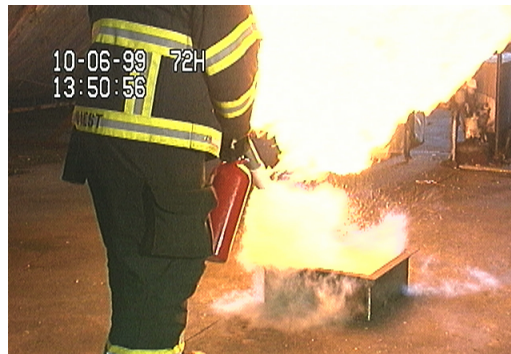
Above, a firefighter extinguishes a fuel pan fire using an extinguisher equipped with the Adiabatic Expansion Nozzle.
