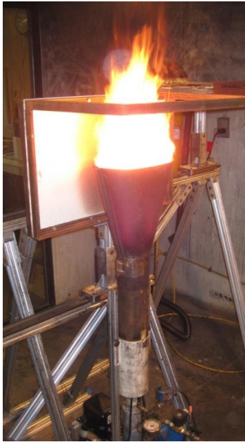
Figure 2. Cargo liner burnthrough test
