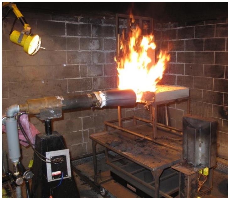
Figure 1. Seat cushion flammability test
