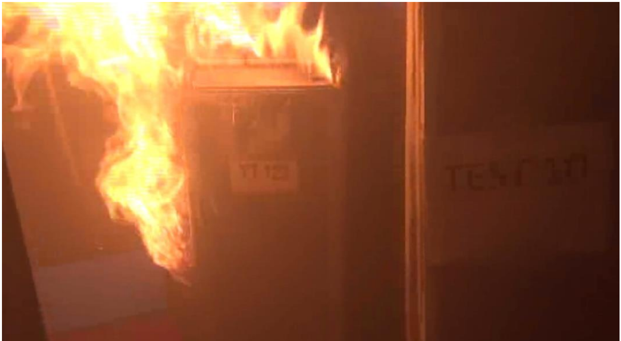
Figure 1. Flames emitted from e-tablets within a closed galley cart
