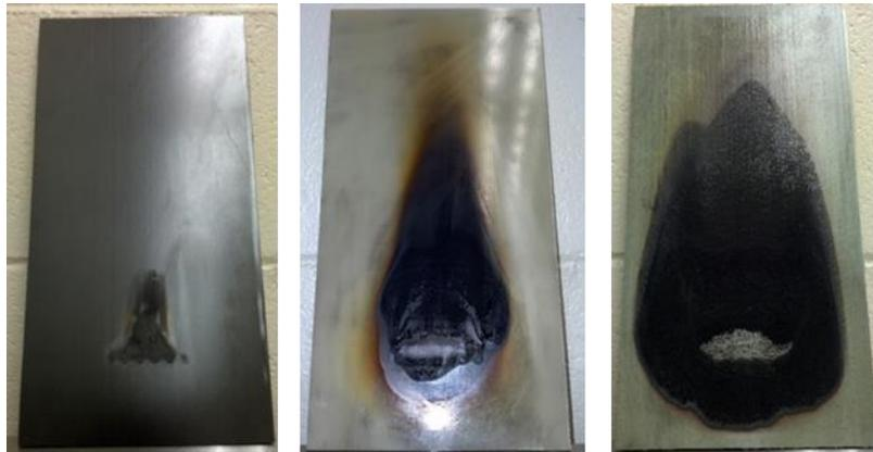
Figure 2. Post-test comparison of burned areas for aerospace carbon/epoxy (L), industrial-grade glass/epoxy (C), and glass/vinylester (R).
