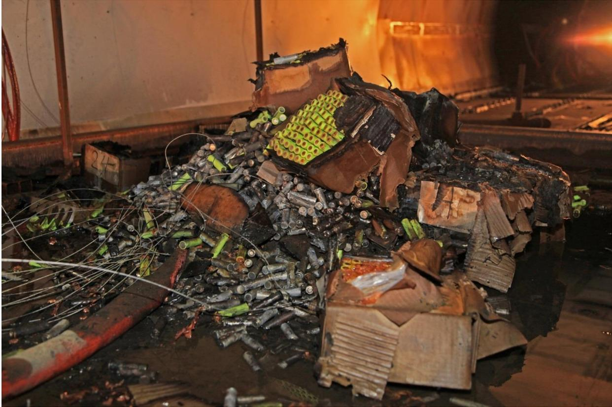
Figure 1 5000 lithium-ion cells after the test was terminated; approximately two thirds consumed in the fire.
