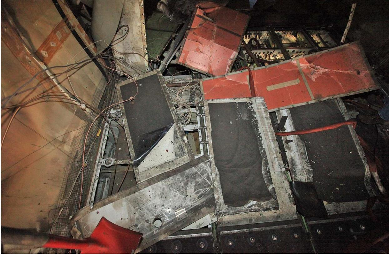
**Figure 1** The ignition of unburned electrolyte hydrocarbons in the mix bay caused an explosion that opened a large hole in the main cabin floor.
