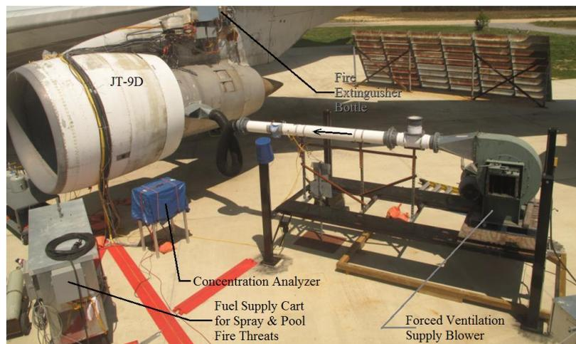
Figure 1. The FAA-owned Boeing 747SP Engine Fire Test Site.
