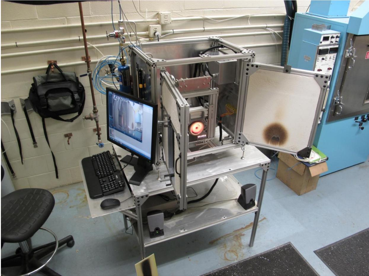
Figure 1. Flame propagation test apparatus
