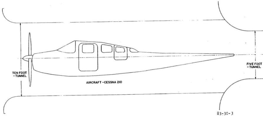
Figure 1. Wind Tunnel Profile with Cessna 210C
