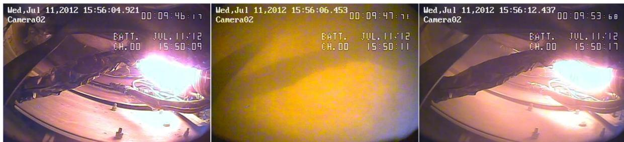
**Figure 2. Pool Fire Imagery in the Engine Fire Zone during the Solid Aerosol Injection and Migration.**
