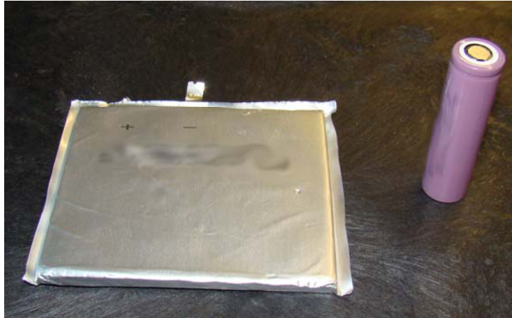
Figure 1. Lithium-Ion Polymer (left) and Lithium-Ion Cells (right)
