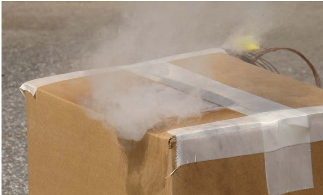
Figure 16. Smoke Venting Through the Flap Seal
