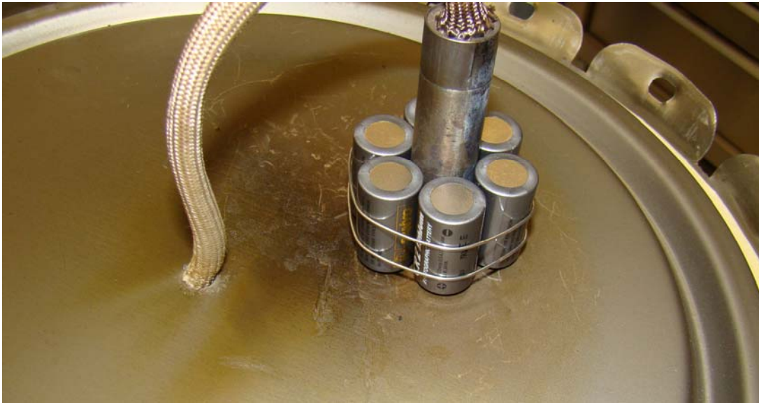
Figure 11. Five-Gallon Pail Test, Six CR2 Cells Wired to the Cartridge Heater
