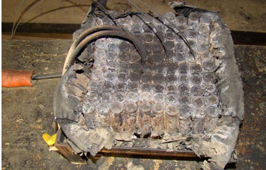
Figure 6. Lithium-Ion Baseline Propagation Posttest
