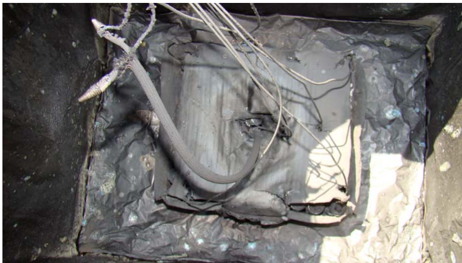
Figure 18. Oxygen Generator Overpack Lithium-Ion Posttest
