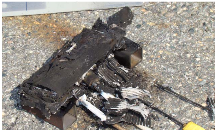
Figure 20. Lithium-Ion Polymer Laptop Battery With Shipping Box Posttest
