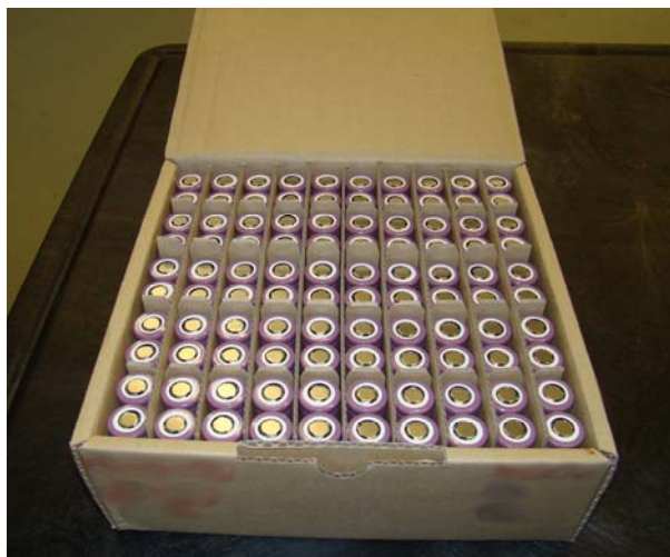
Figure 3. Shipping Box With Interlocking Cardboard Separators for 100 Battery Cells
