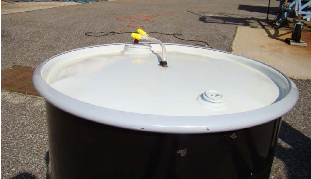
Figure 13. Test 1—Lid Bulge After the Six CR2 Cell Test
