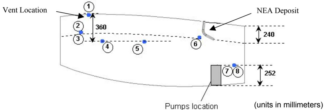
FIGURE 2. SIDE VIEW OF A320 CENTER WING TANK WITH SAMPLE PORT LOCATIONS
