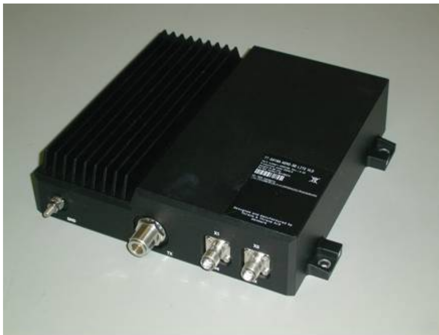
HLD, metal construction with no cooling/vent holes
