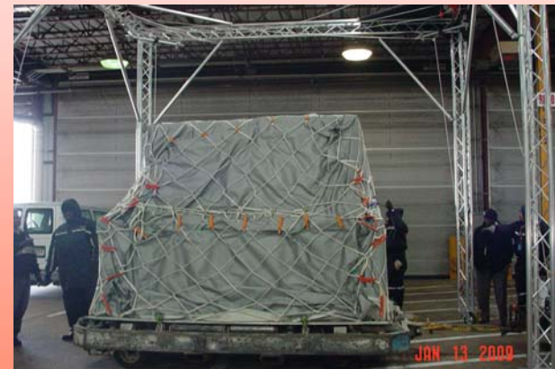
A Fire Containment Cover for palletized freight.
