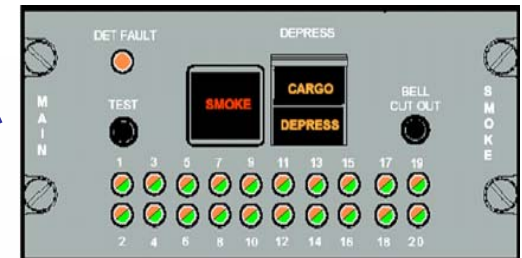
MAIN SMOKE CONTROL PANEL (ON P5)
