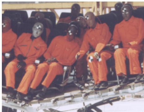
Fig. 19: Change of aisle width during a crash test.
