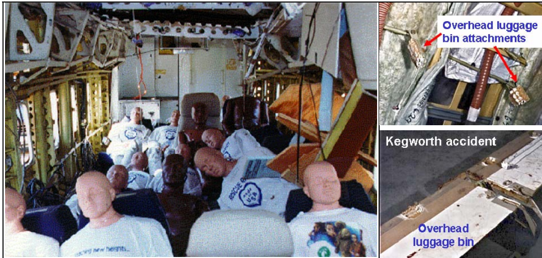
Fig. 18: Failure of overhead luggage bins in test / accident; Source: FAA [8], AAIB [9]
