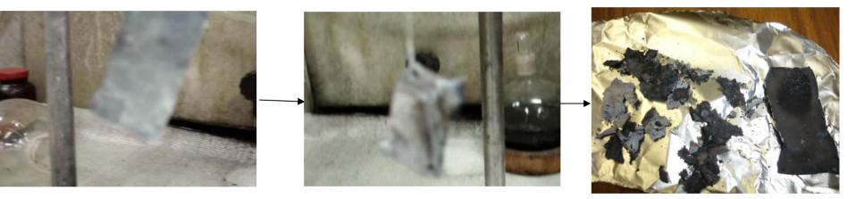
Burning of A12-TiO2 coated camouflage fabric Self extinguish within 25sec. No melt drip Not ASTM standards
