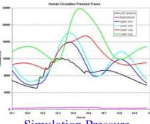
Simulation Pressure Results (With Gravity)
