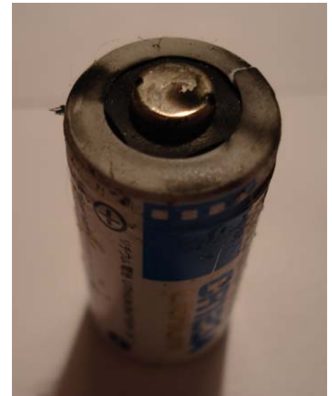
Burnt counterfeit battery
