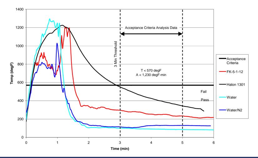
Fire Extinguishing Agents Tested Using the Aircraft Cargo Compartment MPS Standard
