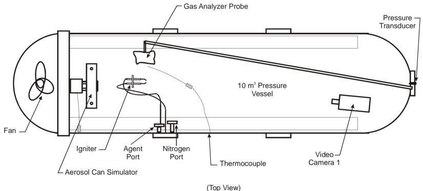
Fire Extinguishing Agents Tested Using the Aircraft Cargo Compartment MPS Standard FIGURE 1. PRESSURE
