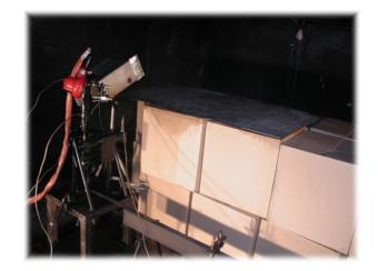
• Heat up simulator to increase pressure in content chamber to 210 psig
