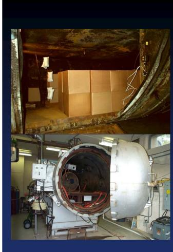
Fire Extinguishing Agents Tested Using the Aircraft Cargo Compartment MPS Standard
