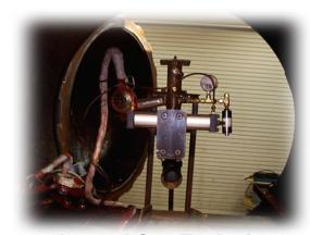
Aerosol Can Explosion Simulation
