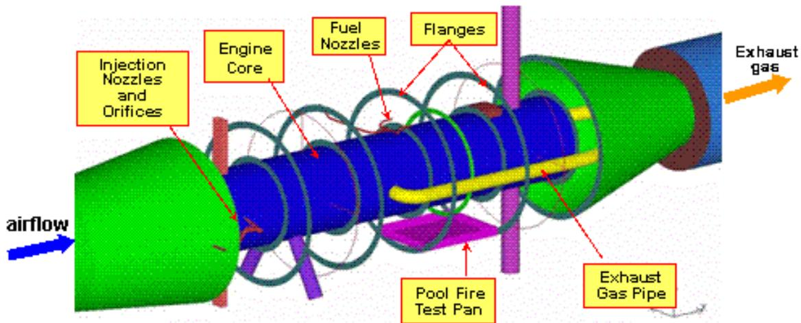
Figure 10: Picture of the Internal Test Section of the FAA Nacelle Fire Simulator
