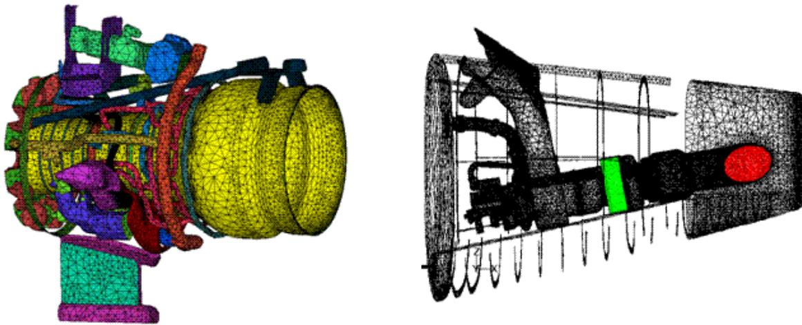
*Figure 8: Unstructured Surface Meshes Inside the Engine Core and APU Compartments*
