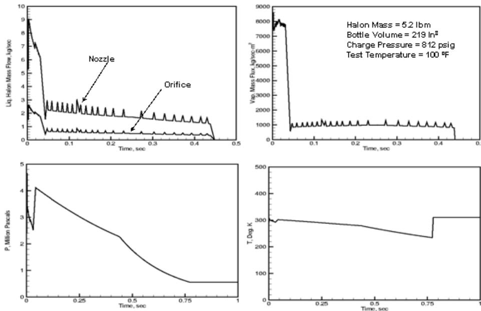
Figure 12: Hflowx Predicted Transient Two-Phase Jet Flow Properties at the Exits of the Injection Nozzle and the Orifice
