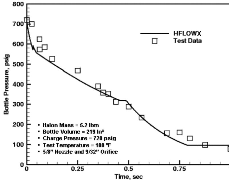
Figure 6: Comparison of Predicted and Measured Bottle Pressure Decay
