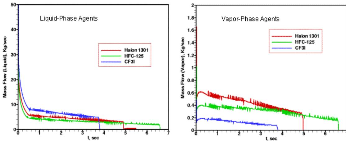
Figure 7: Comparisons of Discharge Characteristics of Firex Agents at Nozzle Exit
