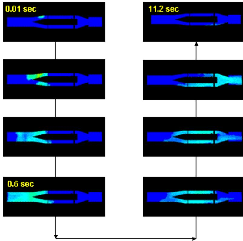
Figure 14: Side View of Jet Injection and Mixing With Counter-Flowing Air Stream
