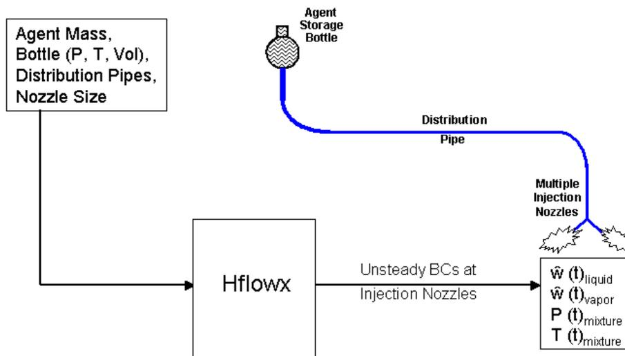
Figure 5: Hflowx Predictions of Flow Properties at the Injection Nozzle Exit
