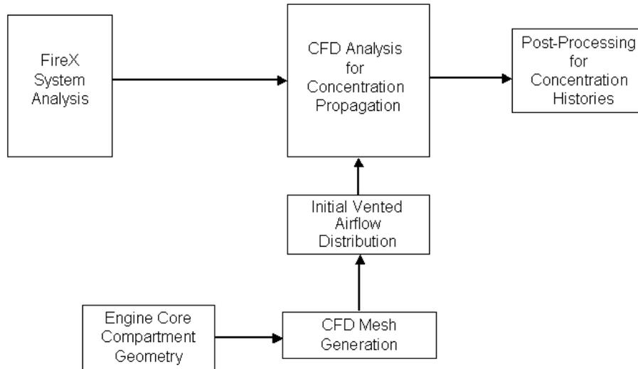
Figure 4: Block Diagram of Elements of the Developed Simulation Process
