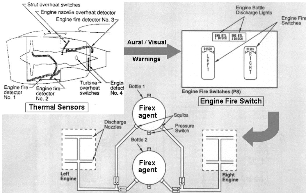
Figure 1: Engine Fire-and-Overheat Detection and Fire Extinguishing
