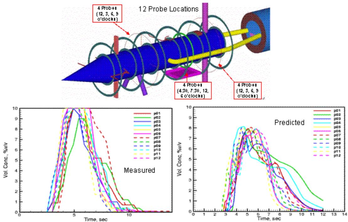
Figure 15: Comparison of Predicted and Measured Concentration Histories at 12 Probe Locations Inside the Nacelle Fire Simulator
