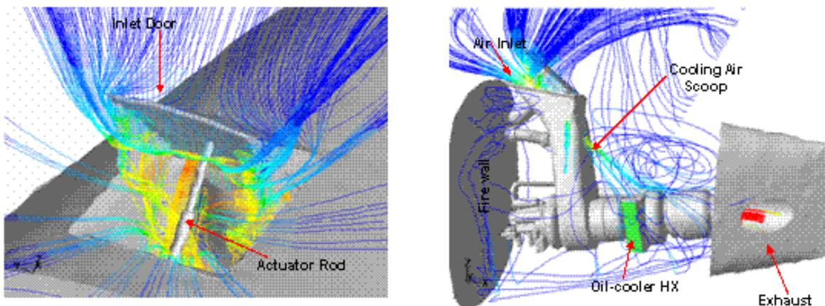
Figure 16: Predicted Path Lines of Cooling Air Inside the APU Compartment
