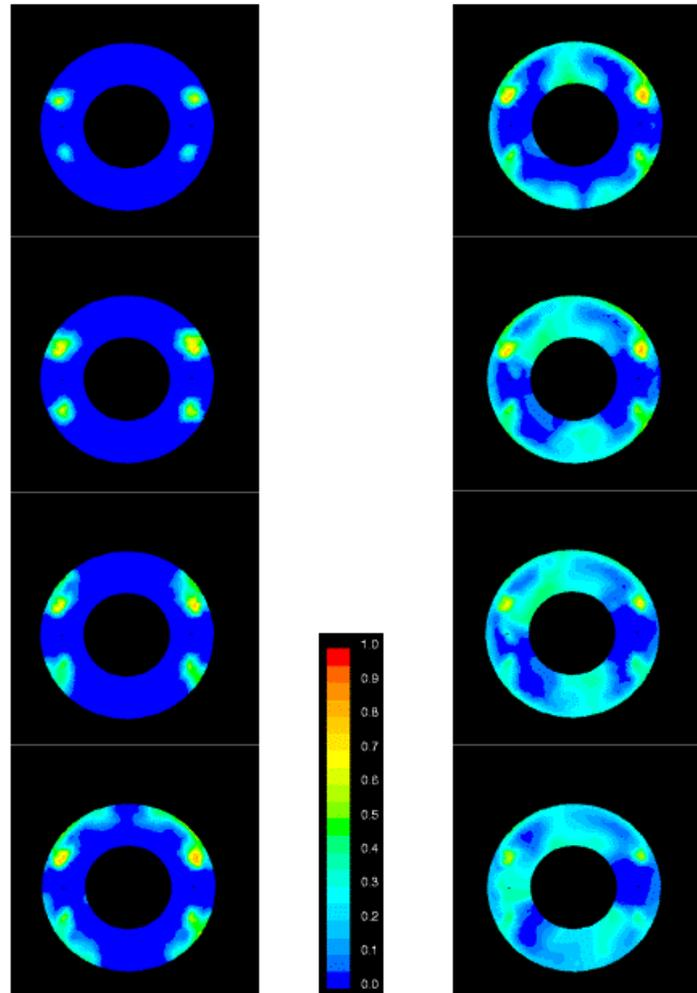
*Figure 13: Front View of Jet Injection and Mixing with Counter-Flowing Air Stream (elapsed time increases from the top to the bottom, from the left to the right columns)*
