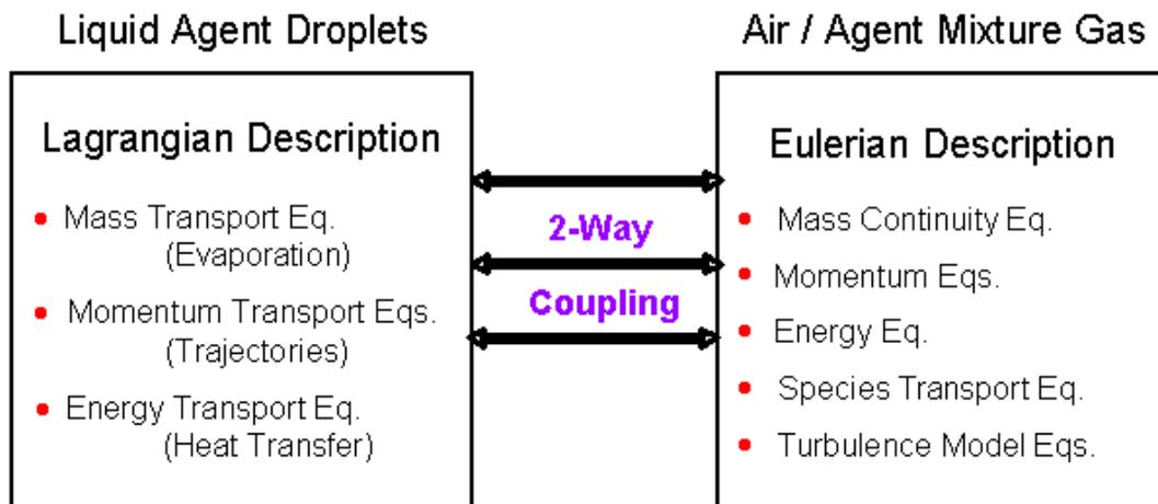
Figure 9: Types of Governing Equations in the CFD Modeling of the Agent Injection and Concentration Propagation Processes
