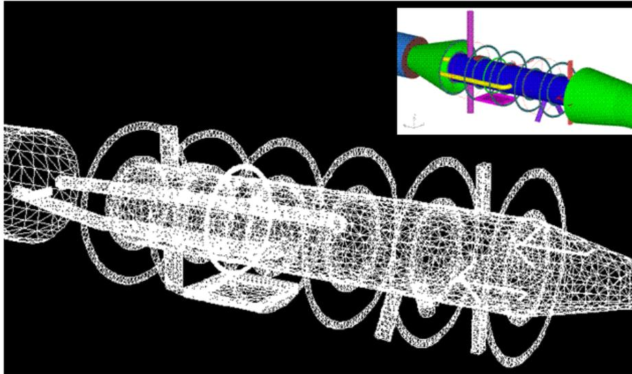
Figure 11: Unstructured Surface Mesh for the Nacelle Fire Simulator
