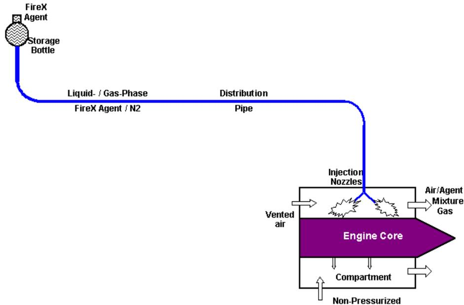
Figure 3: Schematic of Simulated Fire Extinguishing Process
