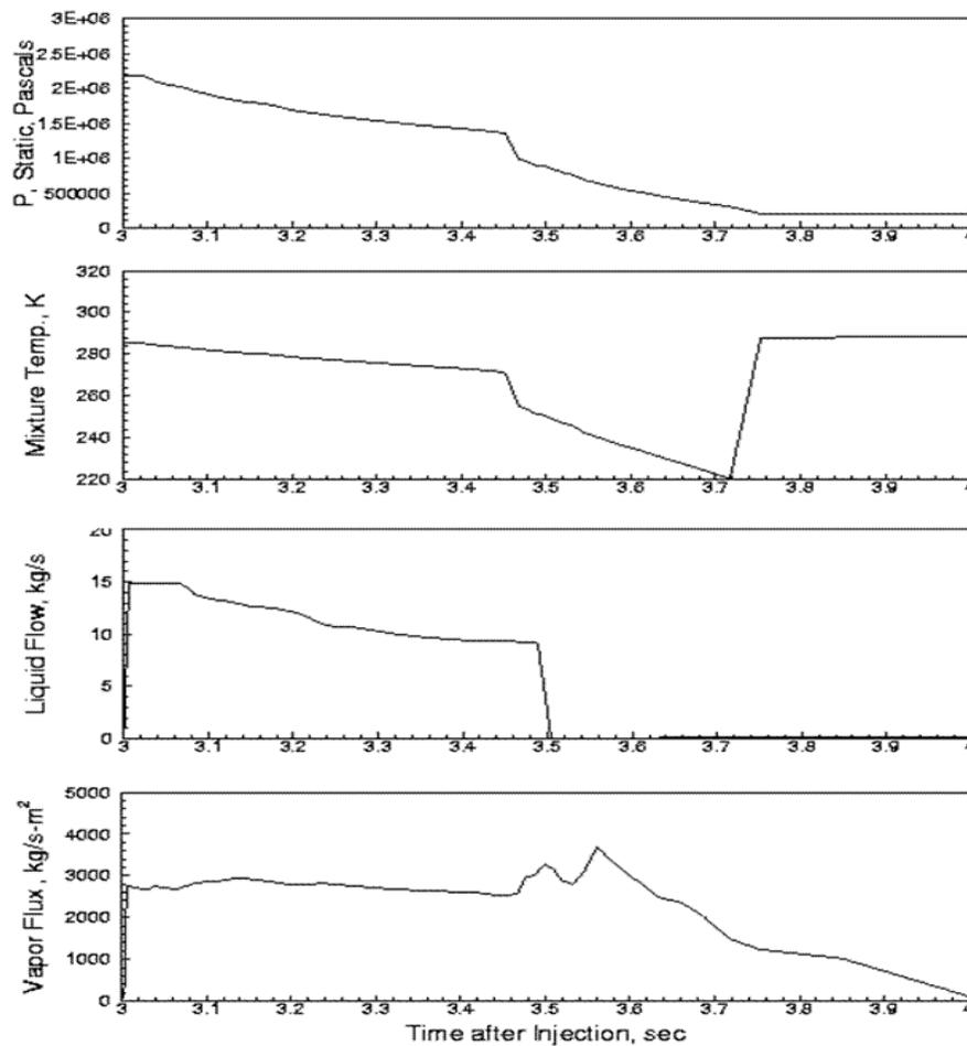
*Figure 17: Hflowx Predicted Transient Two-Phase Jet Flow Properties at the Injection Nozzle Exit*
