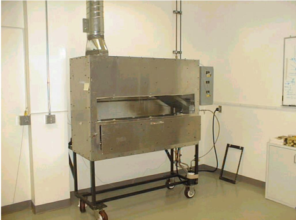
Figure 3. A radiant panel testing apparatus using electric heating elements.
