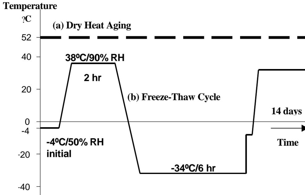
Figure 2. (a) Dry heat and (b) freeze-thaw processes for blanket aging before testing.
