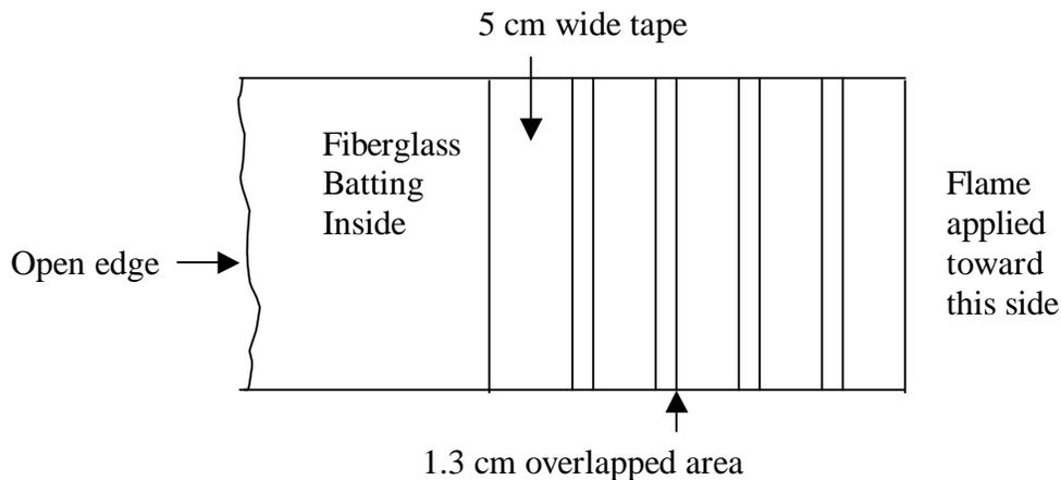
Figure 1. Configuration of a specimen (taped side).
