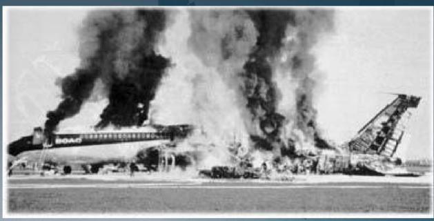
BOAC 707 uncontained engine failure results in in-flight fire, engine separation, then fuel ignition during emergency landing. Five fatalities. April 8, 1968
