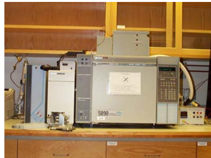
Py-GC/MS: 50~300 \mu g (pyrolysis gases)
