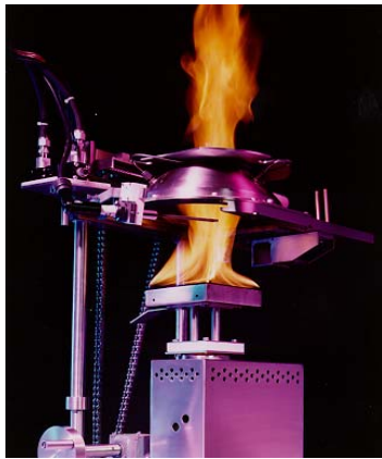
Cone calorimeter: 100g
