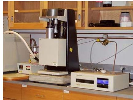
STA (TGA/DSC): 10mg (Thermal decomposition)
