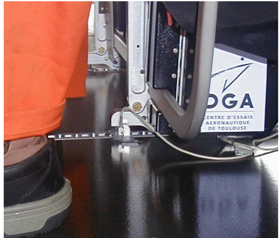
Accelerometers on representative floor
