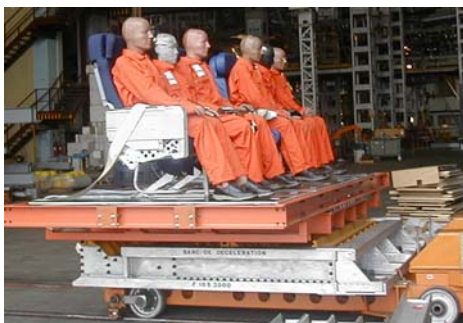
Test rig equipped with two triple tourist seats fitted with different number of rear studs
