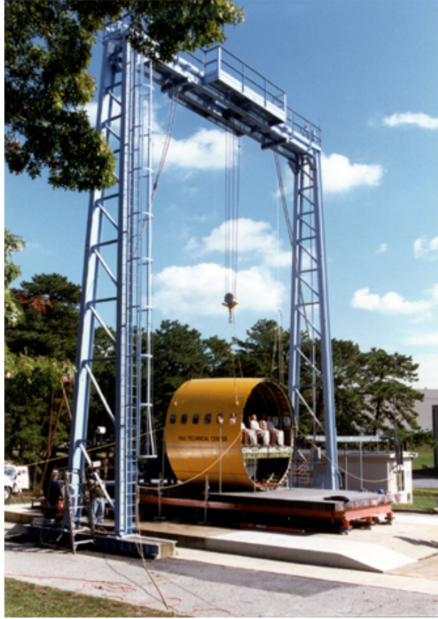
FIGURE 2. DYNAMIC DROP TEST FACILITY
