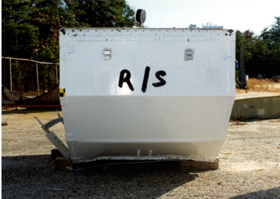
FIGURE A-21. CONFORMABLE AUXILIARY FUEL TANK—RIGHT SIDE
