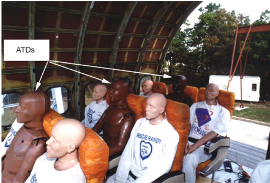
FIGURE 14. ATD LOCATION—RIGHT SIDE
