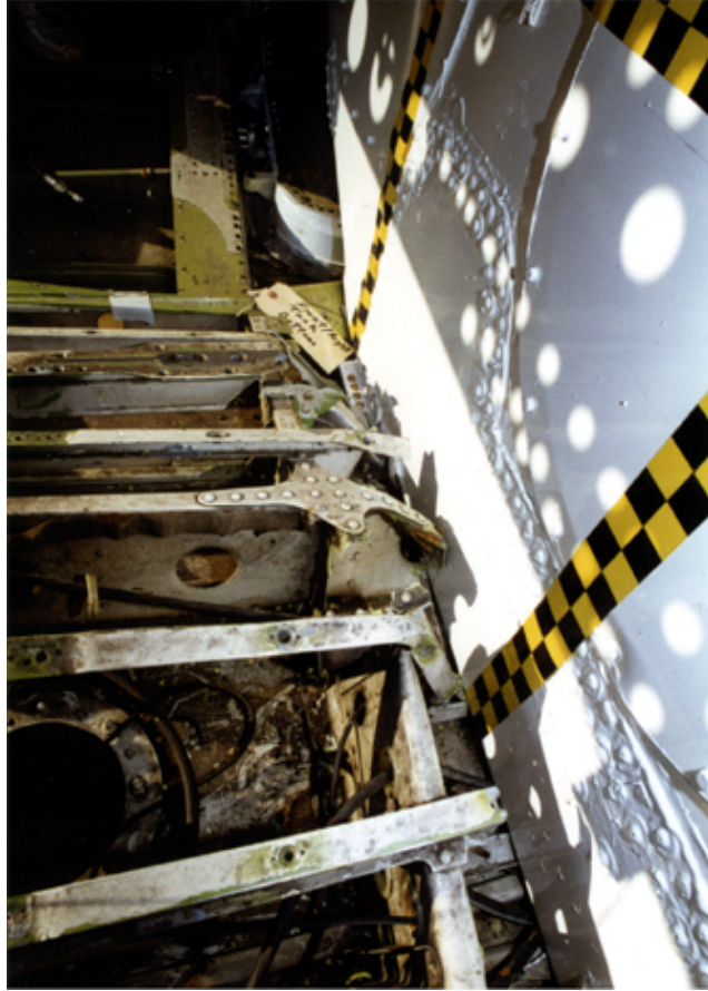
FIGURE 32. FUEL TANK CRUSHING CARGO FLOOR
