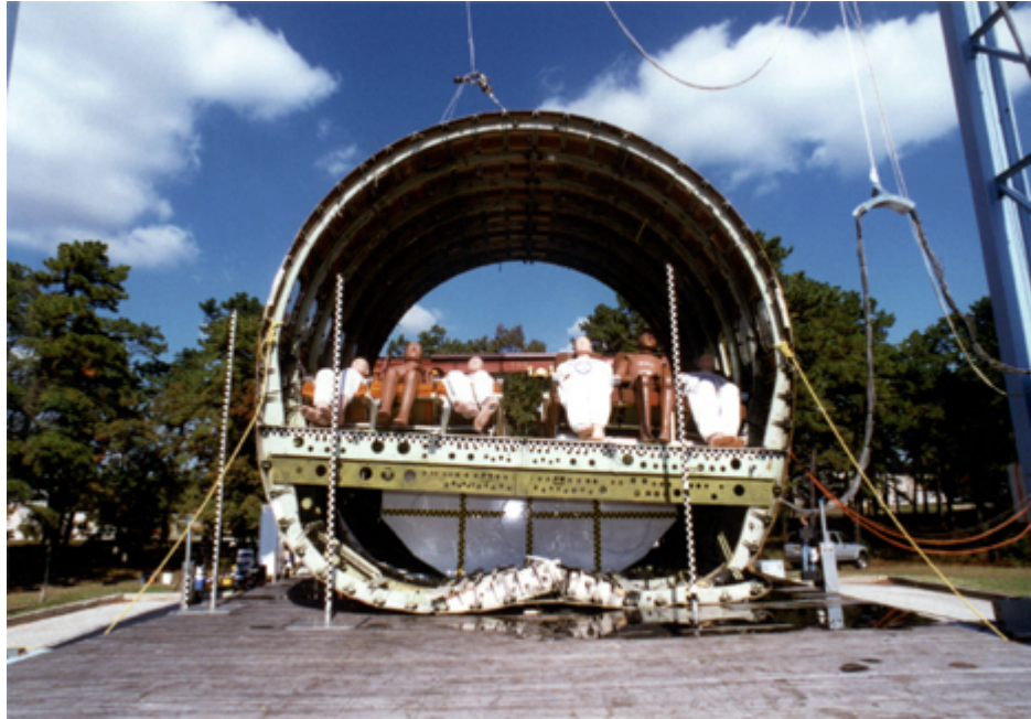
FIGURE 22. FRONT VIEW—LOWER FUSELAGE CRUSH
