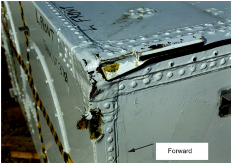
FIGURE A-27. FUEL TANK DAMAGE—LEFT FRONT
