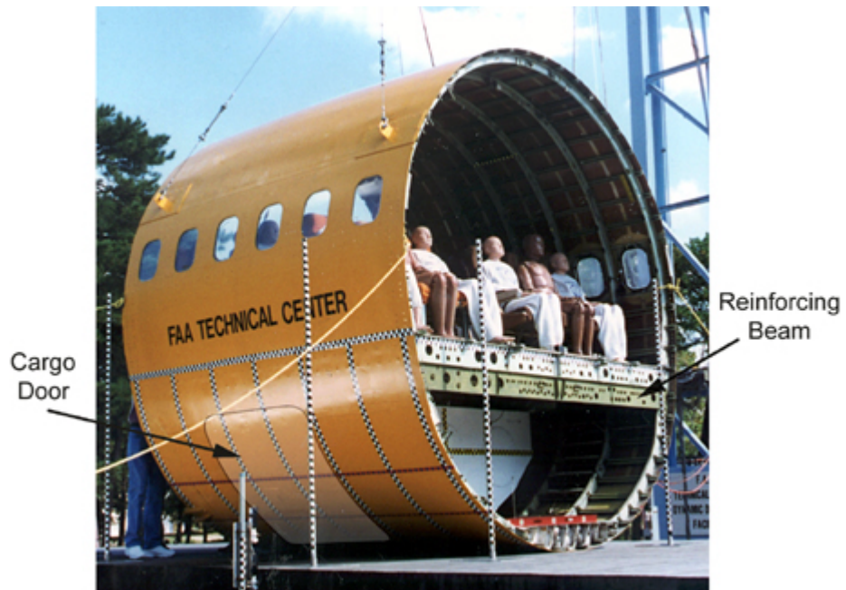
FIGURE 4. TEST SECTION—SHOWING CARGO DOOR AND REINFORCING BEAM
