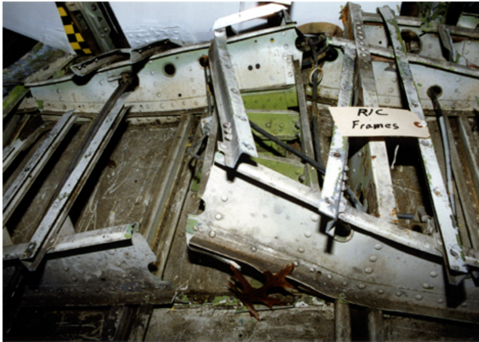
FIGURE A-15. CENTER REAR FRAMES—CARGO AREA
