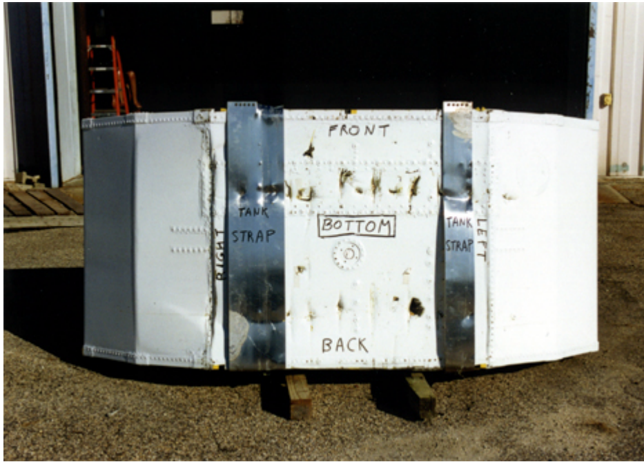
FIGURE A-23. CONFORMABLE AUXILIARY FUEL TANK—BOTTOM
