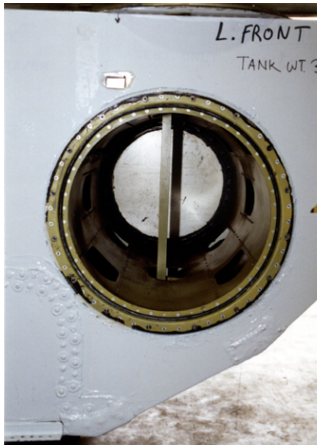
FIGURE A-26. FUEL TANK, STIFFENING MEMBER—LEFT SIDE
