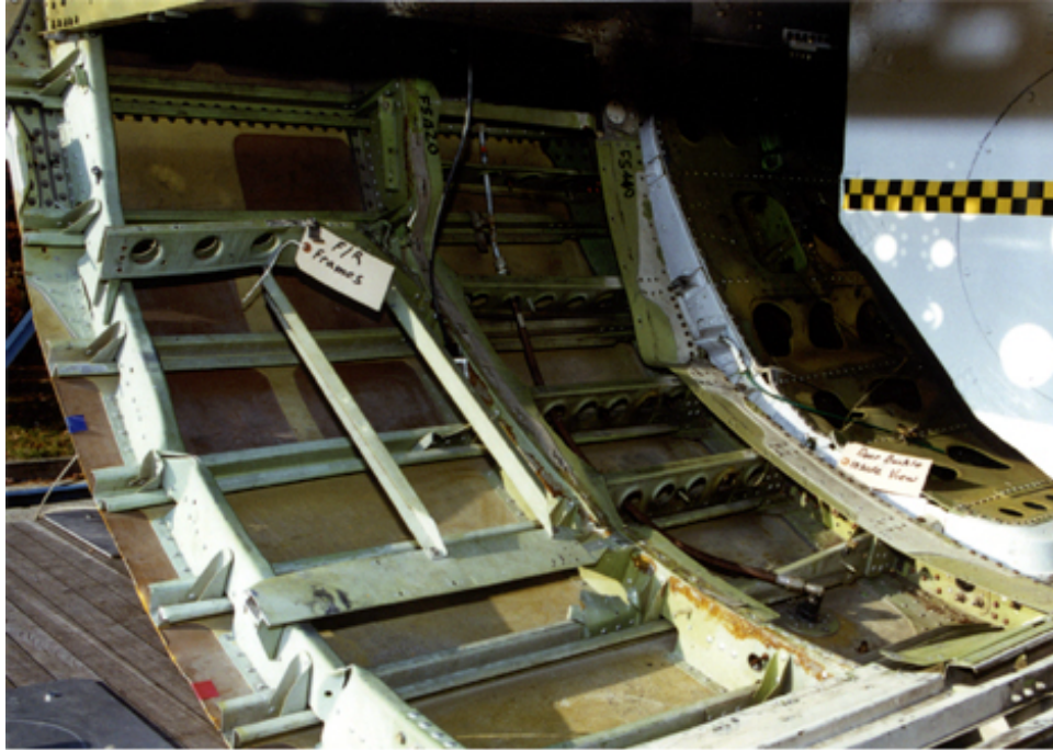
FIGURE A-11. RIGHT FRONT FRAMES—CARGO AREA
