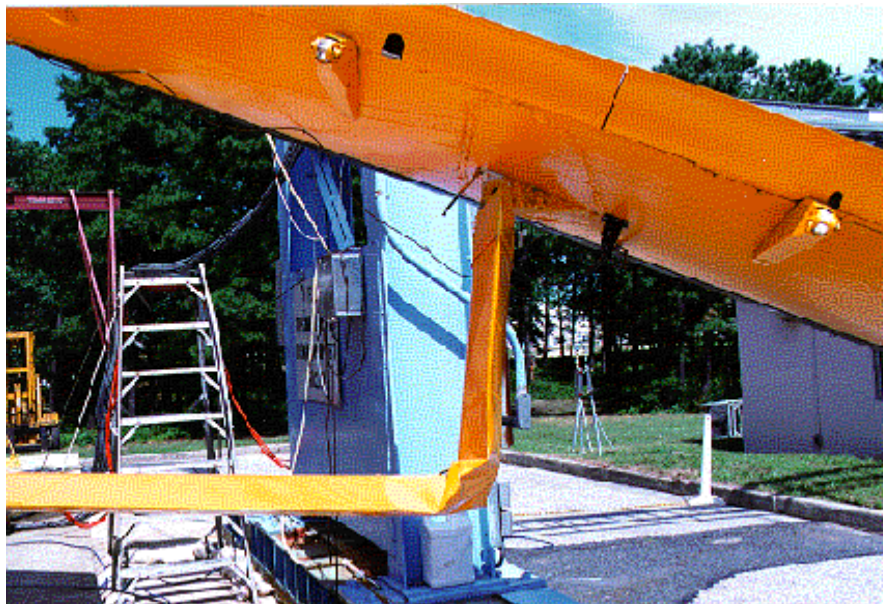
FIGURE 30. COPILOT-SIDE STRUT DEFORMATION POSTTEST
