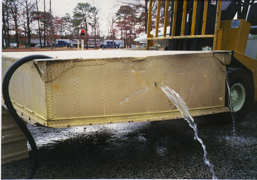
FIGURE 17. CRACK IN CELL 4 PILOT SIDE
