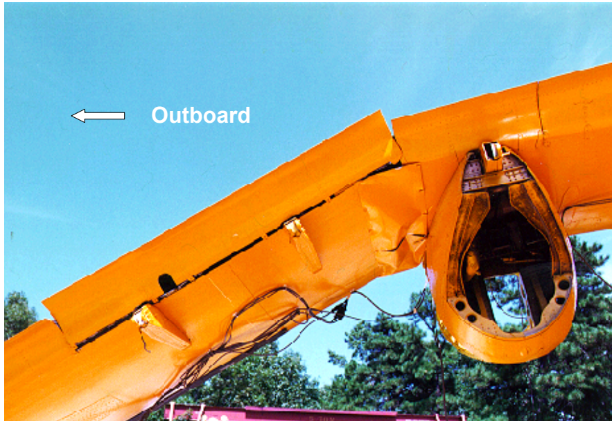
FIGURE 29. PILOT-SIDE WING DEFORMATION POSTTEST
