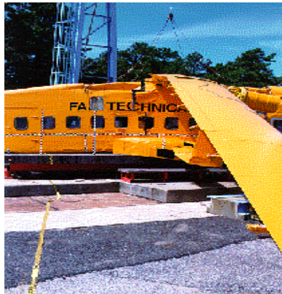
FIGURE 28. COPILOT-SIDE FUSELAGE CRACK POSTTEST
