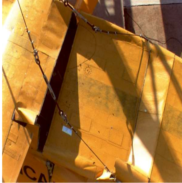
FIGURE 13. FUEL CELL 4 COLLAPSED INTO FUSELAGE
