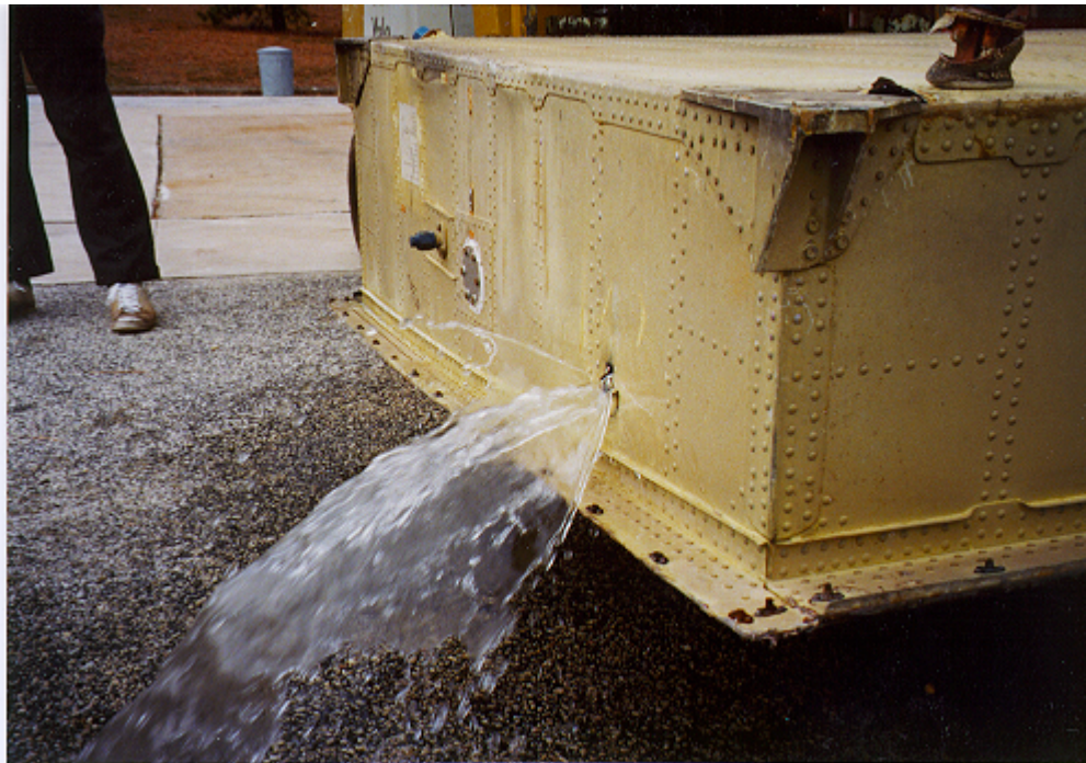
FIGURE 18. CRACK IN CELL 4 COPILOT SIDE
